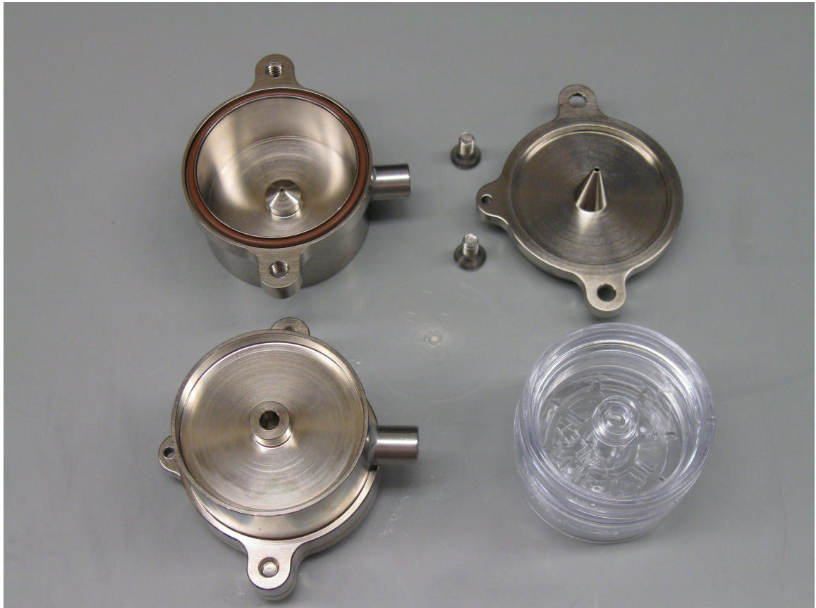
Figure 8. The SADS (lower left) built according to the optimization procedure has the outer shape of 37 mm cassette (lower right) and consists of two pieces, the air nozzle (upper left) and collection probe (upper right).
