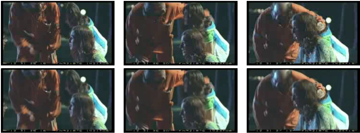
Fig. 14. Several frames of a film compressed with MPEG4 at 128kbps (top row), denoised with AWL (bottom row.)
