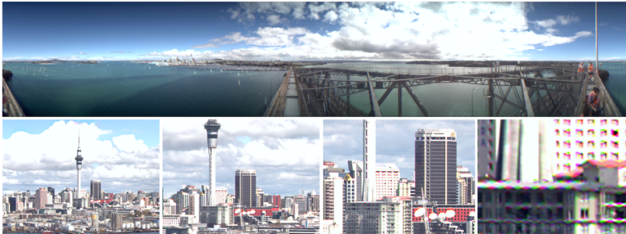
Figure 2.4. Top: a 360^\circ image from Auckland's harbor bridge in 2001 (a rotational scan which took about 4 min; the image is about 350 Megapixel). Bottom, left to right: steps of zooming into the image above, which shows finally (on the right) image jitter which is due to the vibration of the bridge during scanning.
