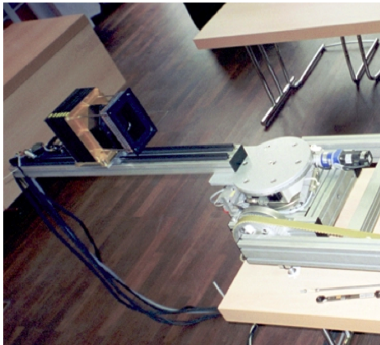
Figure 2.9. Stereo panoramic camera at the Institute of Space Sensor Technology and Planetary Exploration, DLR Berlin, 2000.
