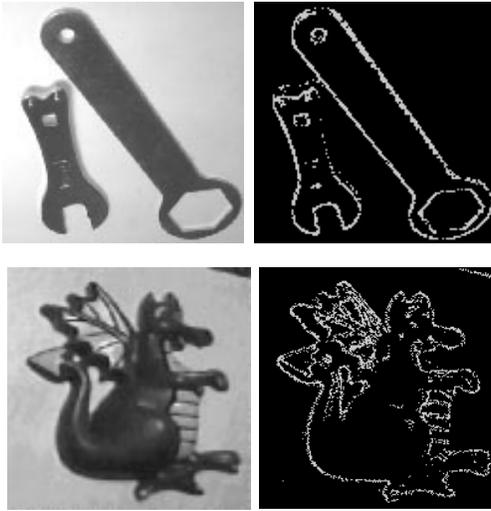
Figure 2: Examples of the affine invariant edge detector (after threshold).
