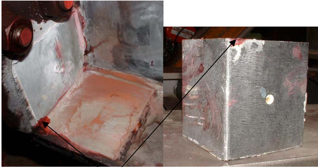
Dye had penetrated a small area at the boundary of the angle
