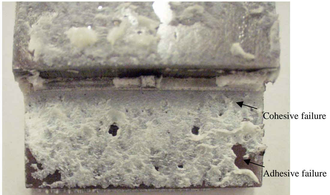
Figure 5.10 Failure mode of a standard baseline specimen (Room temperature cured, tested in lab ambient air, No GPS, bondline thickness t_a= 0.020 in.)
