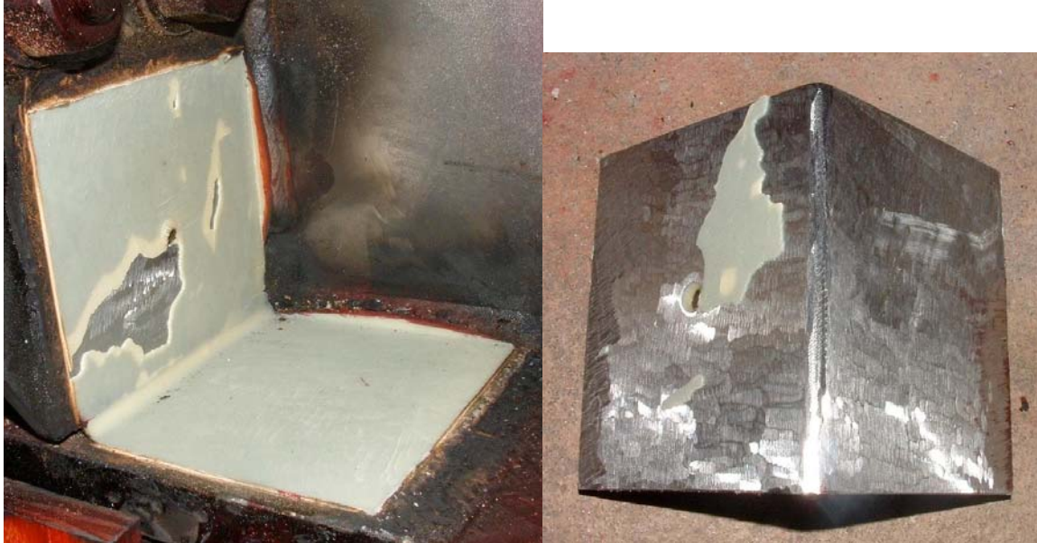
Figure 4.50 Detached angle at web gap NE-1/2
