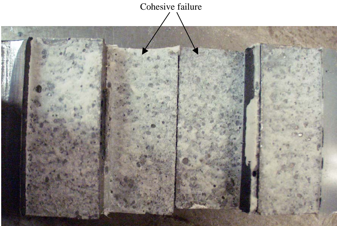
Figure 5.11 Failure mode of a specimen pretreated by GPS (Room temperature cured, tested in lab ambient air, bondline thickness t_a= 0.020 in.)
