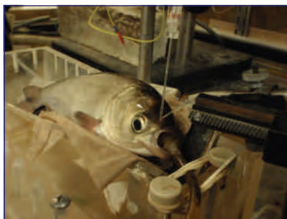
Figure 1. Electro-olfactogram recording (EOG) from the olfactory epithelium of a silver carp while odors are pulsed over its nose. This multi-unit extracellular technique measures olfactory receptor potentials.
