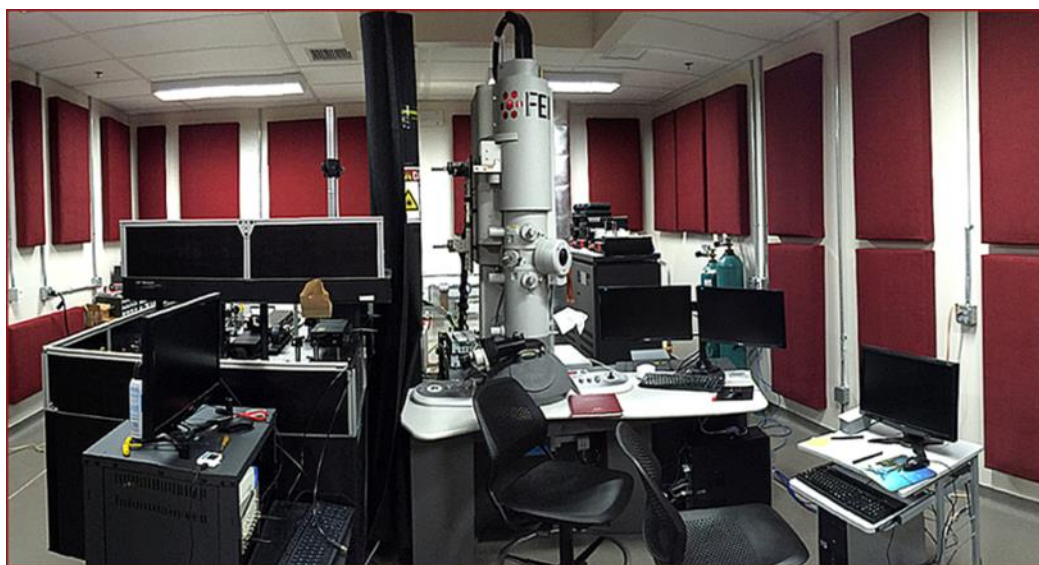
Figure 2.8 A picture of the UEM lab at the University of Minnesota. A FEI Tecnai Femto UEM (right side in the picture) and LASER systems on a Newport optical table (left side in the picture) constitute a major portion of the UEM apparatus.
