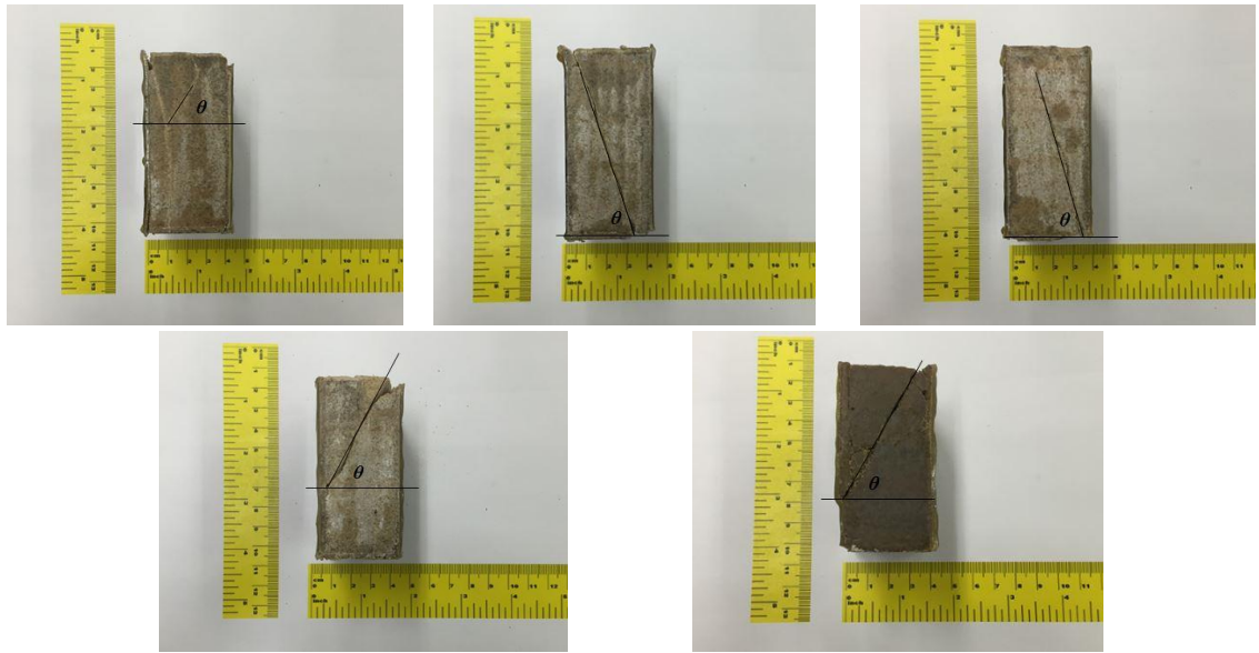
Figure 31: True-triaxial specimens. Top: p = 28.3 MPa. Bottom: p = 56 MPa
