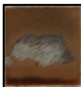
Figure 31: Photo of SiGe film on fused quartz after IPL treatment. IPL parameters: 3 kV, 1 ms, 1250 pulses.
