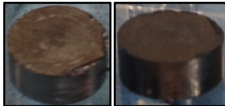
Figure 22: Hot pressed pellets at 30-40% of bulk density.
