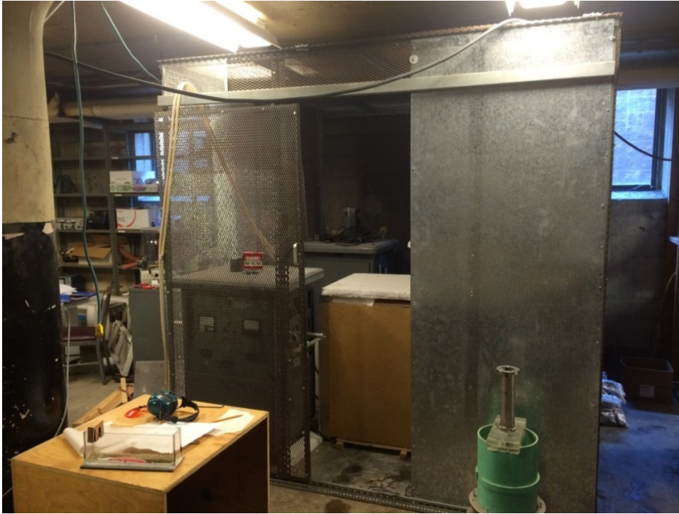
Figure 15: Prototype EPD device at the University of Minnesota-Twin Cities used to process several samples for isotopic analysis.
