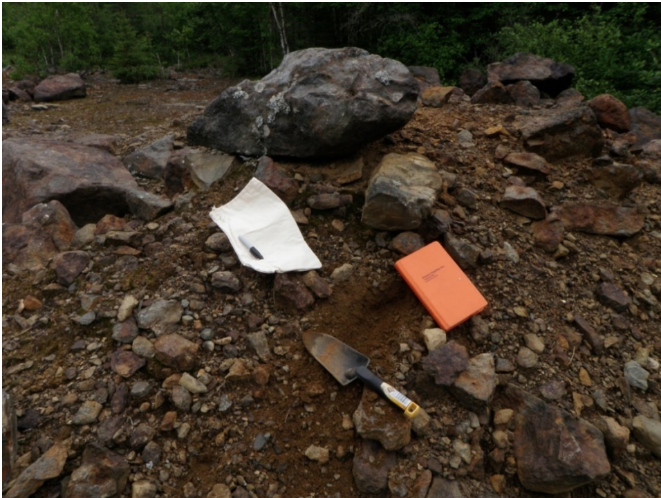
Figure 12: Sampling procedure for till/highly weathered material at the test pit 1 site.
