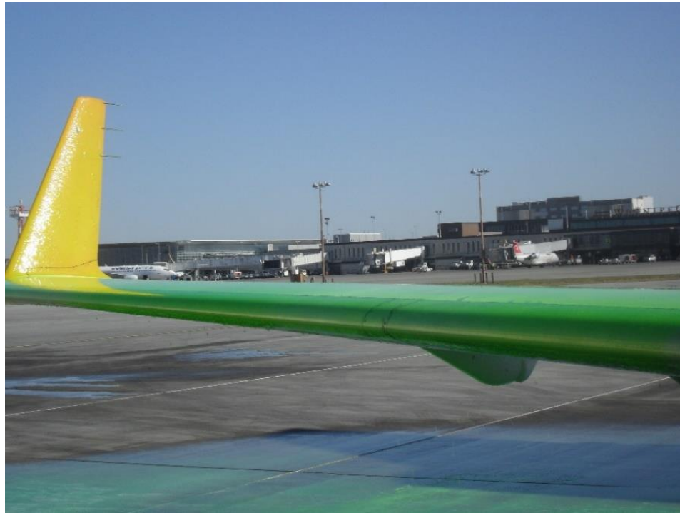
Figure 1.1 Picture of a sufficient coating of Type IV fluid on an aircraft wing.
