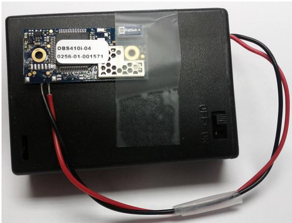
Figure 5-5 A Bluetooth Beacon Prototype Powered by 3 AA Batteries
