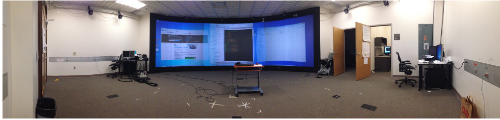
Figure 4.1: Photograph of the display in DDC laboratory at the University of Minnesota used during development of EasyCalibrateVr. The screen forms a semi-circle around the viewer, but curves away from the viewer vertically so that the top and bottom are further away than the center.
