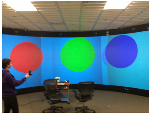
Figure 4.7: Photograph showing the rendering to a calibrated saddle-shaped screen.
