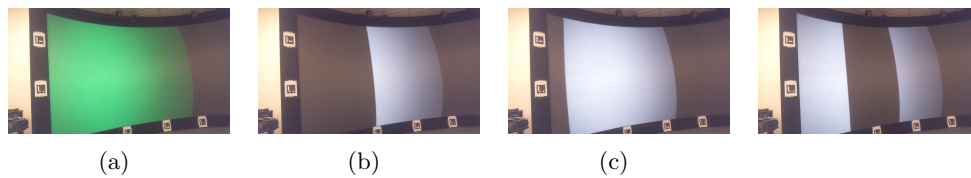
Figure 4.3: Here are some partial images from the graycode pattern shown by one projector. Notice the first frame is an entirely green screen on the projector. This is done so that changing lighting in the room outside the projector screen is not mistakenly identified as part of the graycode pattern.
