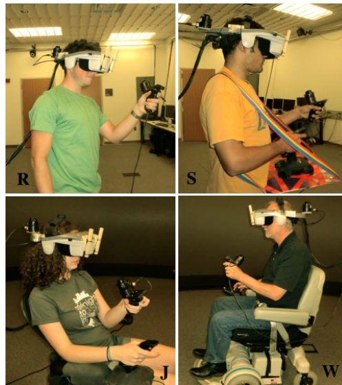
Figure 5.2: Photographs of the different locomotion methods: real walking ( R ), joystick translation while standing ( S ), motorized wheelchair ( W ), and joystick translation while sitting ( J ). Figure from [129].
