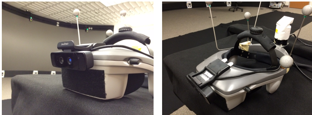
Figure 3.17: This figure shows the final mounting of the Senz3D camera to the NVIS HMD. The camera is attached using double-sided tape and is upside down in order to place it as close as possible to the wearer's line of sight.
