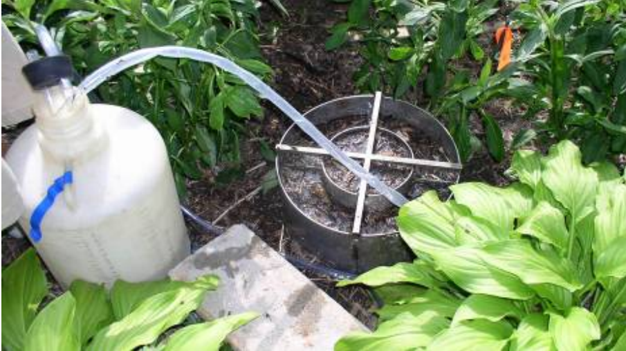
Figure 4: Double-ring infiltrometer with Mariotte system
