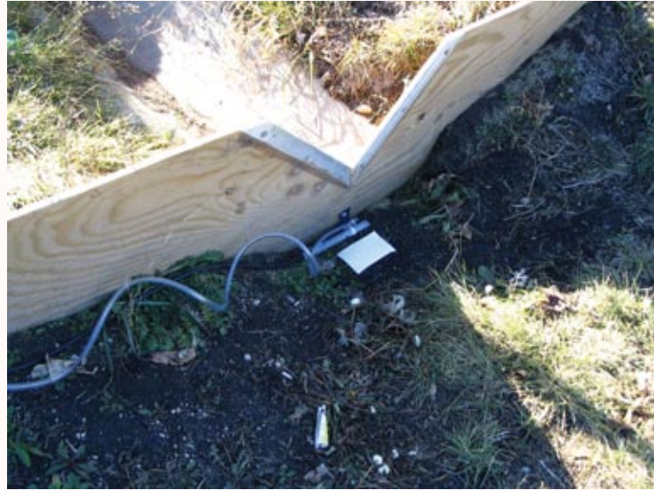
Figure 5.7: Pressure probe for flow measurement and sampling tube for pneumatic sample collection placed at a weir to measure stormwater inflow.
