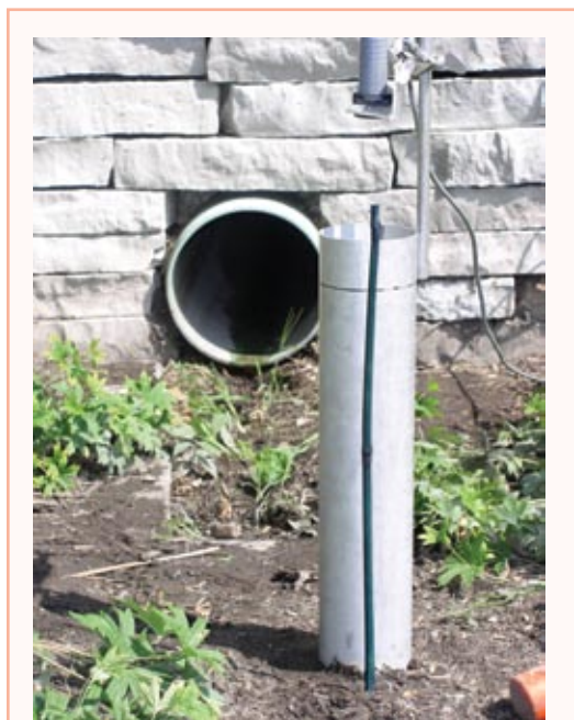
Figure 3.3: Permeability testing with a Modified Philip-Dunne Permeameter in St. Paul, MN.
