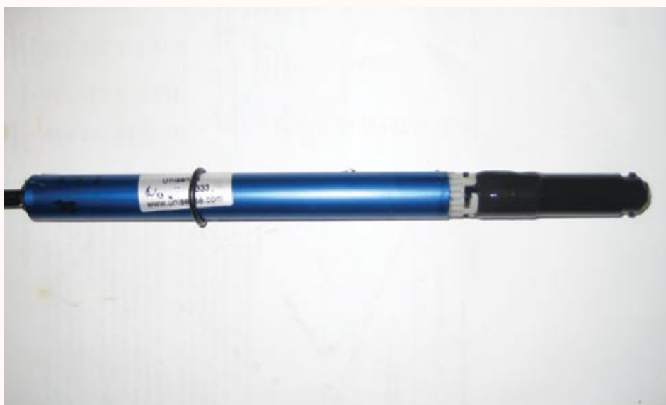
Figure 5.5: In situ probe for measuring nitrate concentration manufactured by Unisense (approximately 8 inches (20.32 cm) in length).
