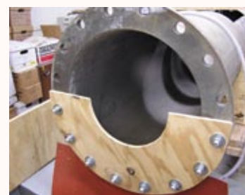
Figure 4.9: Circular weir schematic (top) and test setup photo (bottom, St. Anthony Falls Lab).
