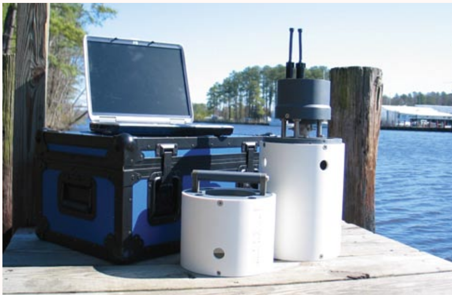
Figure 5.6: MicroLAB in situ nutrient measurement system for nitrate, phosphate, ammonia and silicate systems manufactured by Envirotech Instruments.
