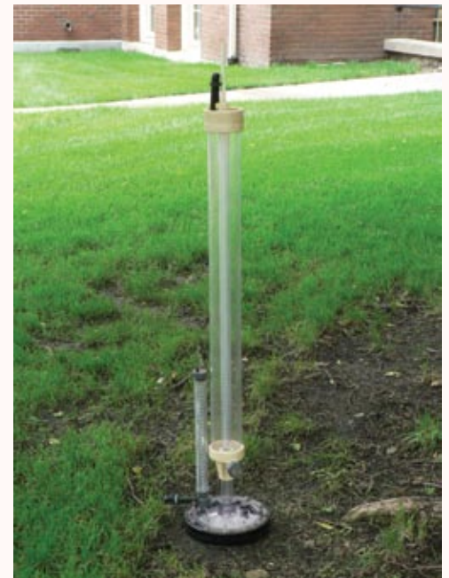
Figure 4.19: Illustration of the Guelph tension infiltrometer
