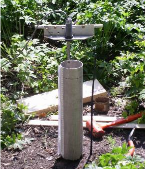
Figure 5: Modified Philip-Dunne Permeameter with ultrasonic sensor
