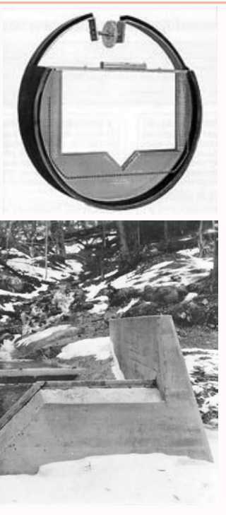
Figure 4.4: V-notch compound weirs in pipe application (top, http://www.geneq.com/catalog/en/vw.htm ) and for open channel flow (bottom, http://www.usbr.gov/pmts/hydraulics_lab/pubs/wmm/chap07_13.html ).
