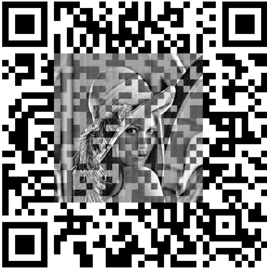
Figure 5: QR code created with the sub-pixel method using 32 pixel modules and a scale factor of k = 6
