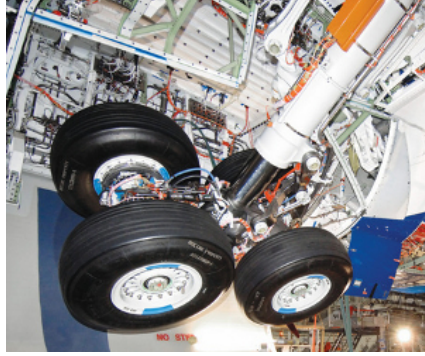
Figure 1: Hundreds of flexible conduits in the landing gear of an airplane.
