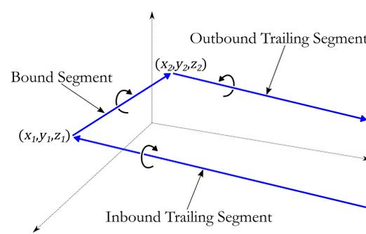
This project's lifting-line simulator can solve a system of equations to yield the strengths of these vortices, with the results thus far agreeing with established data.
