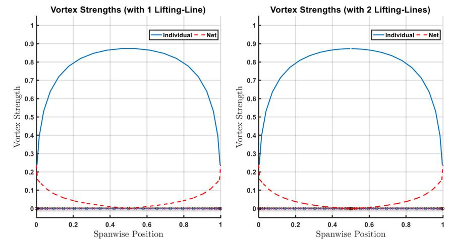
The close agreement between the two cases validates the simulator's handling of multiple lifting surfaces. The decrease in net strength toward the middles of the spans is the result of interior trailing horseshoe segments overlapping and therefore counteracting each other's effects. The cancelling effects result in the greatest vorticity being located at the wingtips, providing consistency with other experimental results (such as those from the NASA study shown in the *Background* section).
