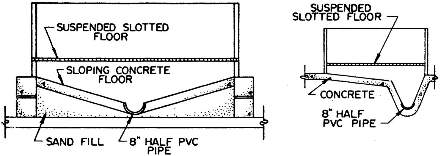
Figure 4. V-shaped gutter (left) and J-shaped gutter (right) under suspended slatted floors.
