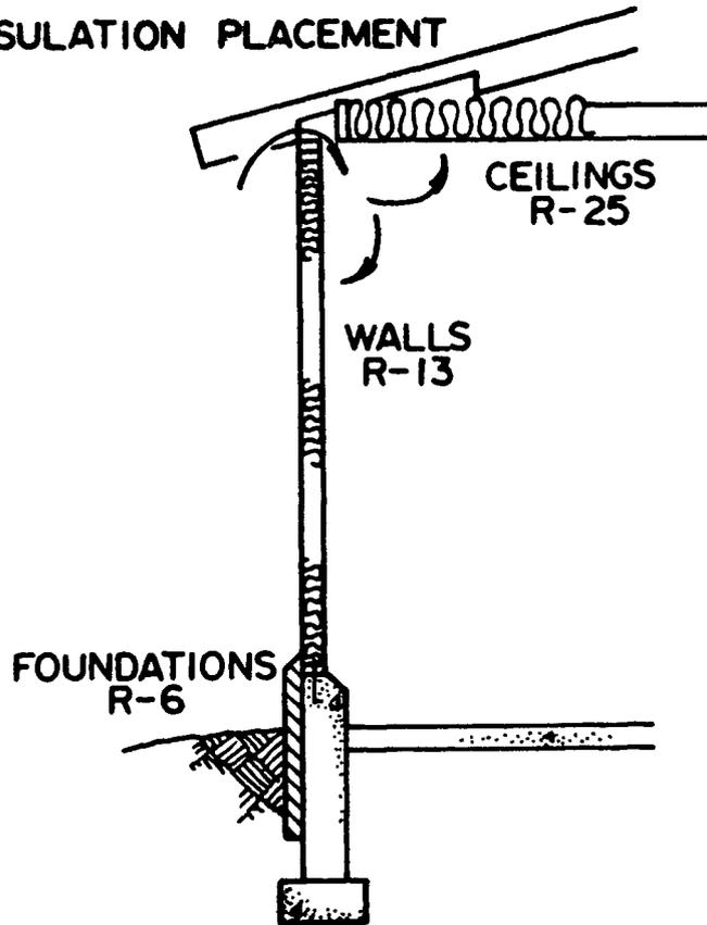
Figure 8. Recommended placement and amount of insulation in a mechanically ventilated barn.
