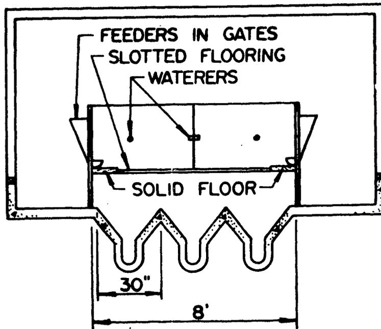
Figure 3. Y-shaped gutters used with raised nursery decks.
