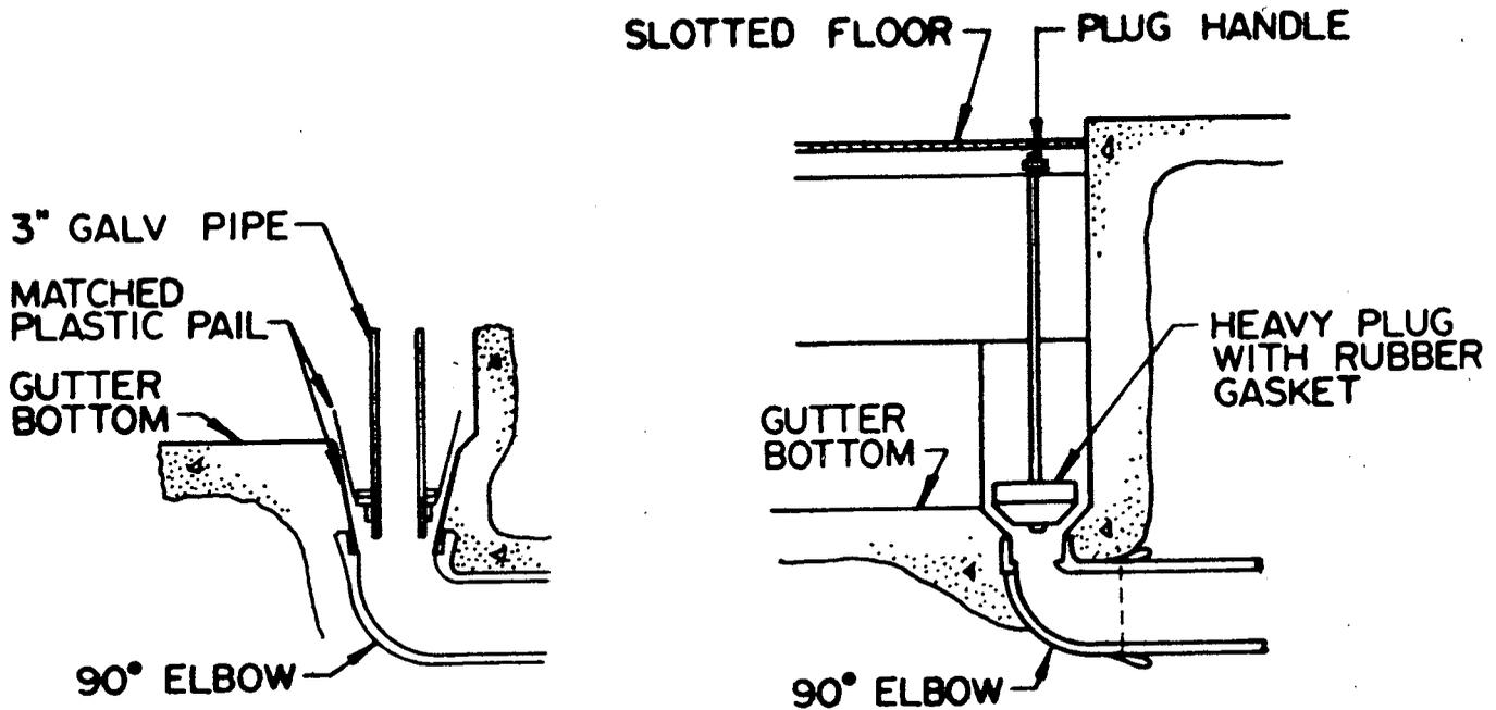
Figure 7. Plastic pail (left) and weighted gasket (right) plugs used in gravity-drain systems.
