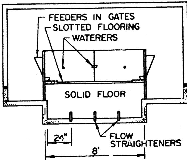
Figure 5. Wide rectangular gutter, with flow straighteners, under suspended flooring.
