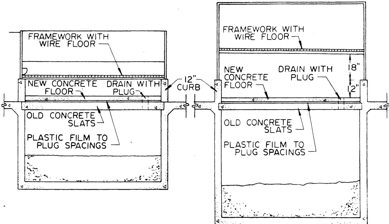
Figure 11. Raised farrowing crate conversion over old pit.
