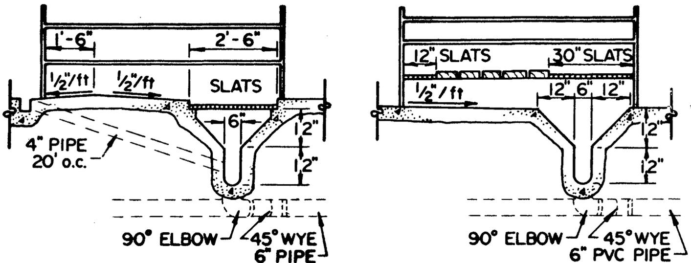
Figure 2. Y-shaped gutters used with floor-level (left) and raised (right) farrowing crates.
