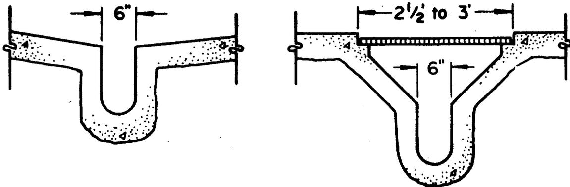
Figure 1. Deep, narrow gutter (left) and Y-gutter (right).
