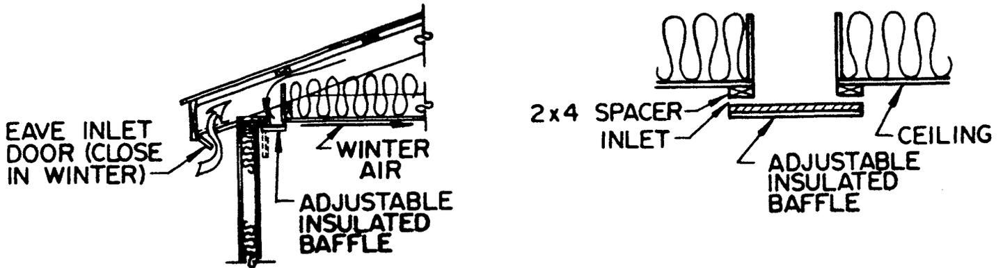
Figure 10. Slot (left) and ceiling (right) air inlets.
