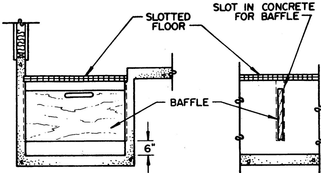
Figure 6. Baffles placement in rectangular gutter to aid in solids removal.
