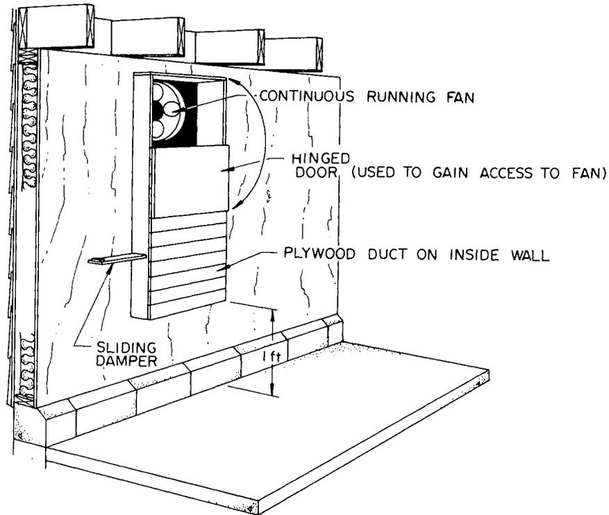
Figure 9. Plywood duct built around the continuously running fan.
