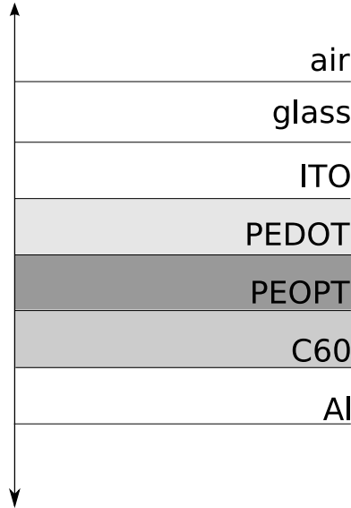
Figure 1: Qualitative arrangement of layers in solar cell
