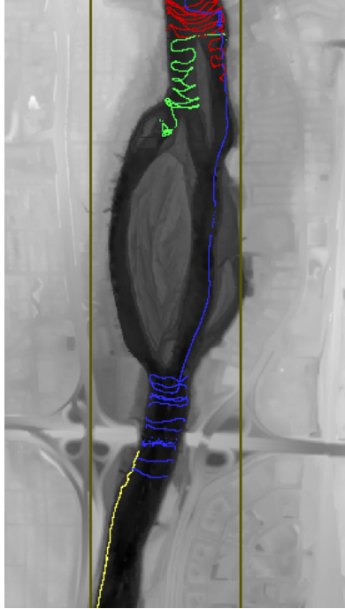
Figure 16: Velocity field measurements were carried out by ADCP along the colored lines: May 16 th (yellow path), June 13 th (red path), July 14 th (green path), and July 31 st (blue path) of 2014.
