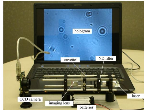
Figure 2. The digital inline holography setup is shown above.
