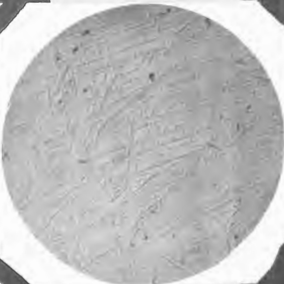
PHOTOMICROGRAPH 42. STEEL VI. held 15 minutes at 1050° C and quenched.. X 800 Martensite and austenite.
