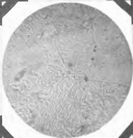
PHOTOMICROGRAPH 30. Steel III. held 15 minutes at 1000° C. X 800 Martensite.
