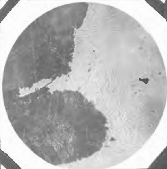
PHOTOMICROGRAPH 5 STEEL V. original C 1.06% Mn 1.45% Troostite and mar- tensite.
