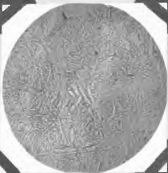
PHOTOMICROGRAPH 33. STEEL IV. held 15 minutes at 900° C. and quenched. X 800 Martensite.
