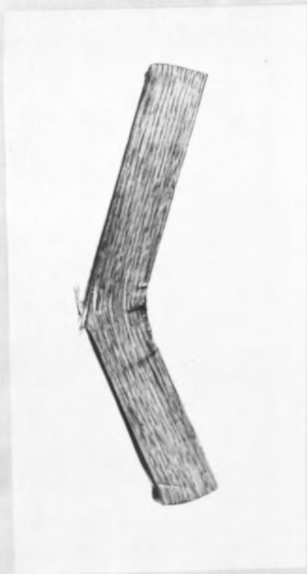
Fig. 41. Steamed oak column showing three zones, tension compression and a central neutral zone. Scale 1/3
