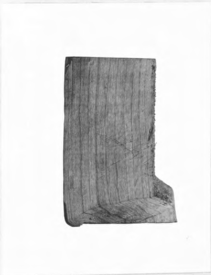
Fig. 23.. Maple block showing an extremely wide shear zone due to a continued application of pressure. Note also the fracture pattern in the center of block.
