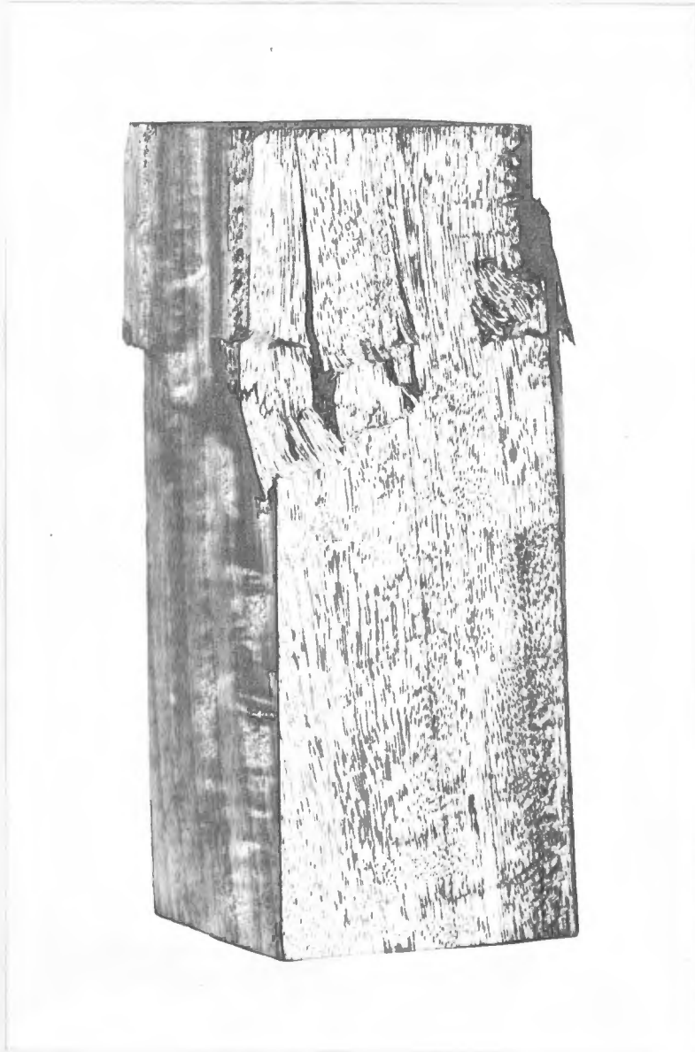
Fig. 1. Satin-wood block deformed under a pressure of 40,000 lbs. Note the brecciated zone of shearing. Scale full size.
