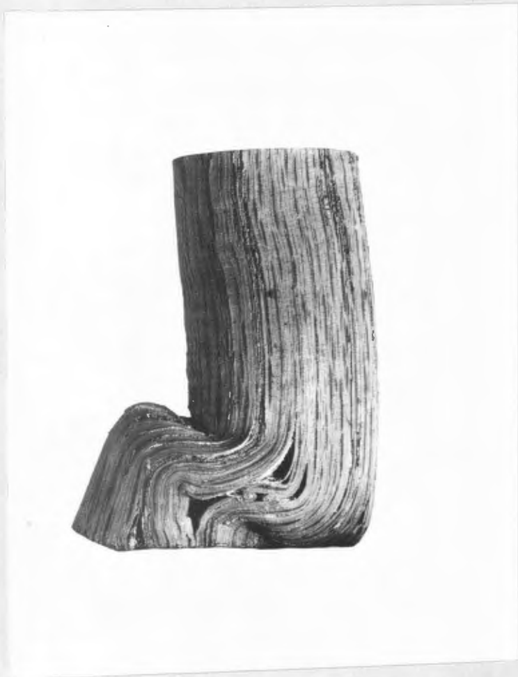
Fig. 27. Steamed oak cylinder. Note the overturn folds within the shear.
