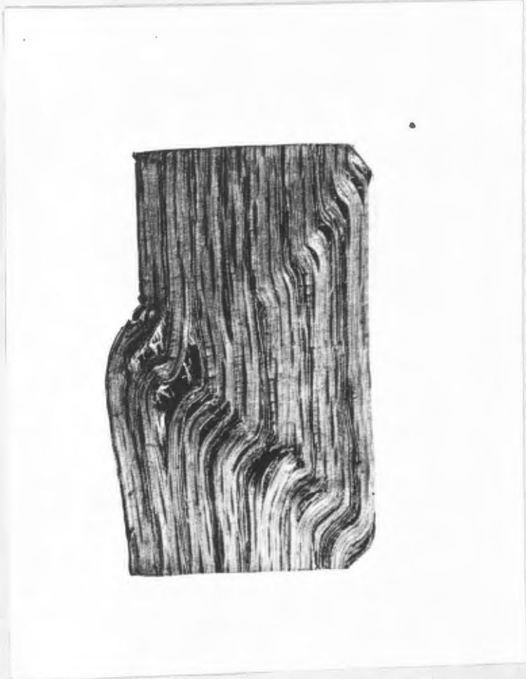
Fig. 25. Steamed oak block. Note the width of shears and the absence of any sharply flexed fibres.
