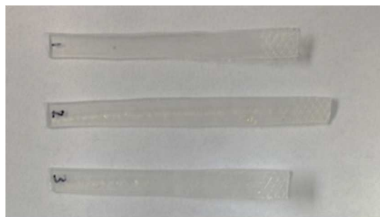
Figure 6.5. Capillary coextrusion LLDPE/PLA bilayers after adhesion testing. Samples are about 6 mm wide and 1 mm thick.
