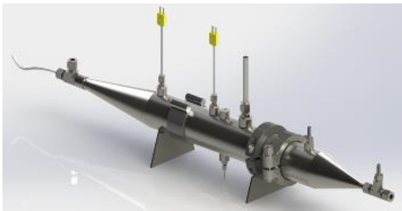
Figure 5.3 Design of the oxidation-dilution tunnel
