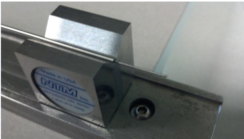
Figure 7 Pin gage or mandrel held down by magnetic V-block and holding driveshaft specimen in place
