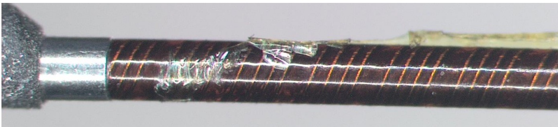
Figure 20 Observed abrasion on the polyimide outer layer after life testing
