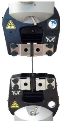
Figure 11 Driveshaft gripped in pneumatic grips.
