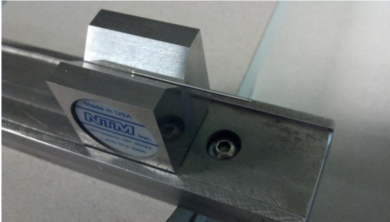
Figure 6 Driveshaft specimen placed into V-block
