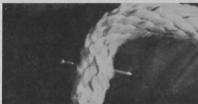
Figure 2. Technique for inserting nail into rope. A. Nail perpendicular through rope.
