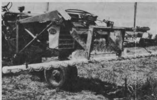
Figure 1. Completed and mounted pipewick applicator.
