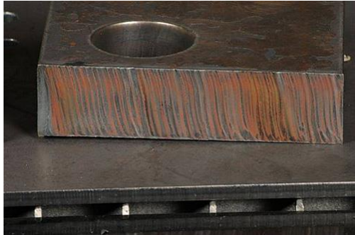
30 mm (1.18 in) plate cut with a plasma torch
