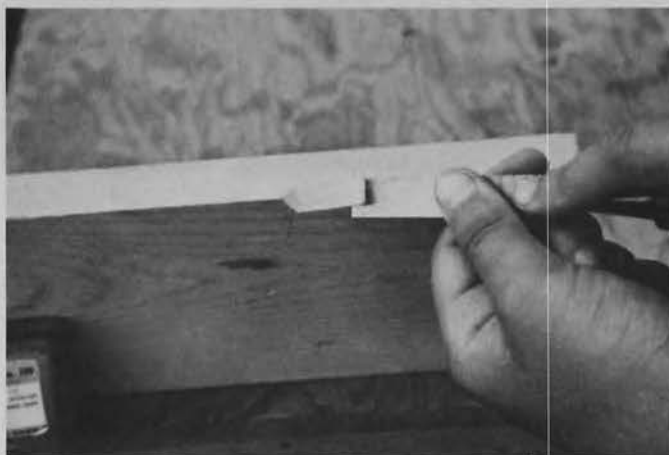
A clamp to hold the chisel or plane iron for grinding.
