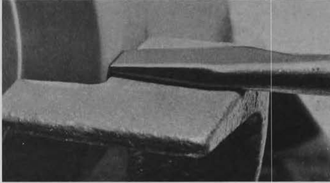
Because of the low angle, the block plane is used for fine work and end grain.
