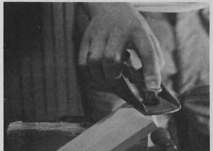
The block plane works well to cut chamfers and bevels.
