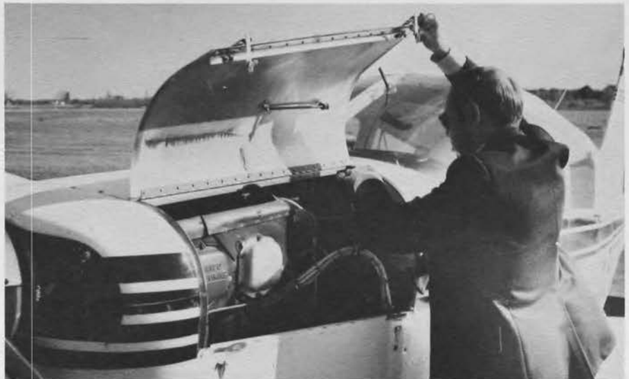
This four cylinder reciprocating aircraft engine develops up to 150 horsepower. Inspection and maintenance standards for airplane engines are much greater than for automobile engines.
