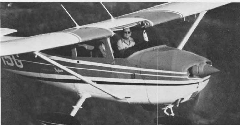
This is a high-wing monoplane which means it has the wing attached to the top of the fuselage. Other monoplanes may be mid-wing or low-wing. (Photograph by Stephan Wilkinson, courtesy of "Flying" magazine.)
