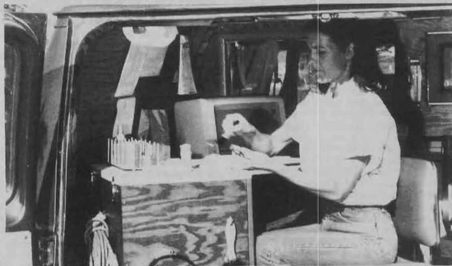
Technician Rebecca Hayes prepares a sample for analysis in the NIR mobile forage testing van.
