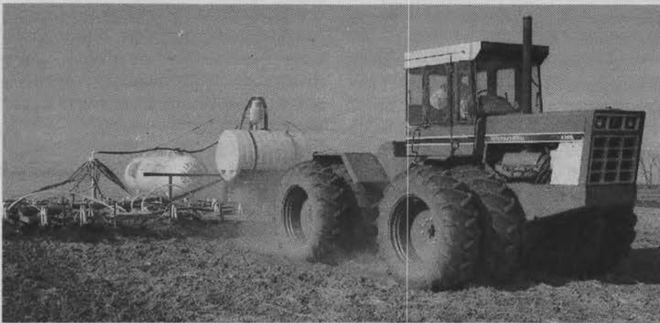
An example of precision farming. Changing anhydrous ammonia applications "on the go" yields economic and environmental benefits. (photo by Don Breneman)
