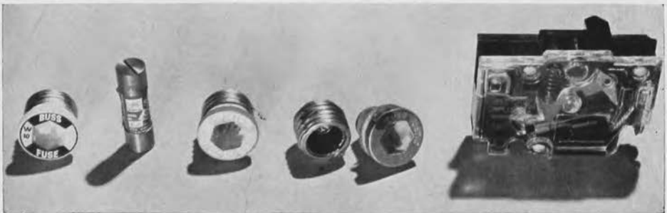
Fig. 6. Various types of fuses are available for farm use. From left to right: plug fuse, cartridge fuse, delayed action fuse, nontamperable delayed action fuse with adapter, and a circuit breaker.
