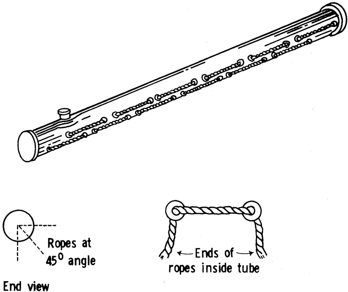
Figure 1. Outside view of rope-wick applicator showing the placement of ropes which act as the wicks. The tube was 3-inch PVC piping capped on the ends. The ropes were soft braided nylon marine rope. The holes in the tube for the ropes were 5/8 in. in diameter and spaced alternately 8 and 2 in. apart. The applicator was constructed as outlined by J. E. Dale, Plant Physiologist, Southern Weed Science Laboratory, USDA, AR-SEA, Stoneville, Mississippi.
