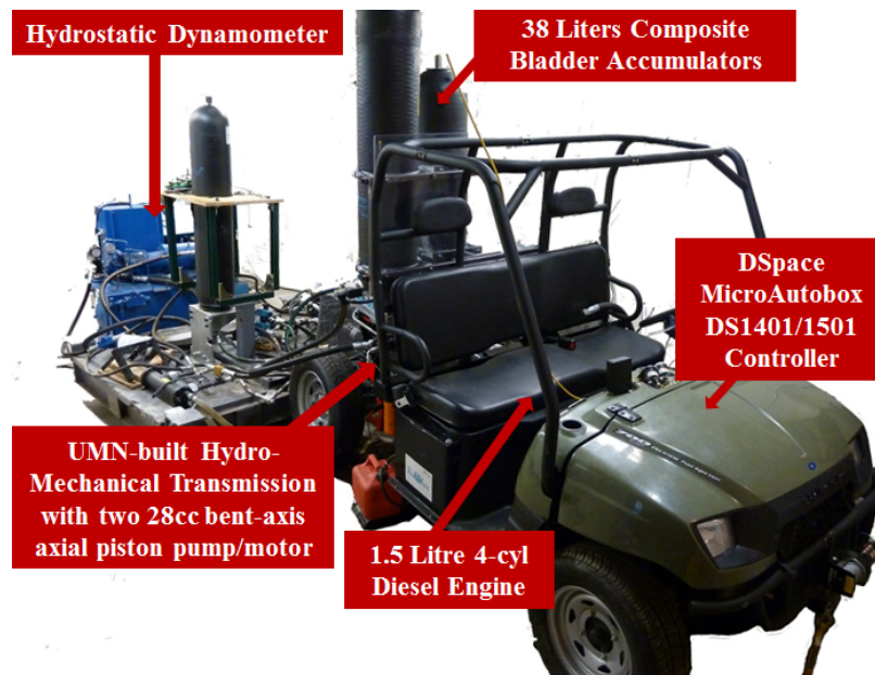
Figure 5.1: Hydraulic Hybrid Passenger Vehicle and hydrostatic dynamometer built by CCEFP at University of Minnesota.
