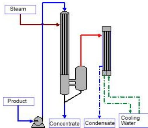
Figure 9: 1 effect evaporator plant layout (Source: GEA Group AG, 2013)
