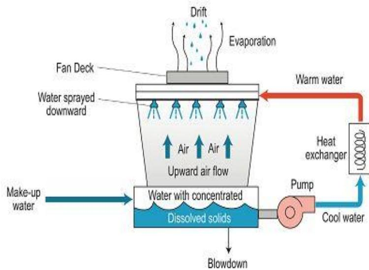
Figure 7: A typical cooling tower setup (source: R.L Deppmann, 2012)
