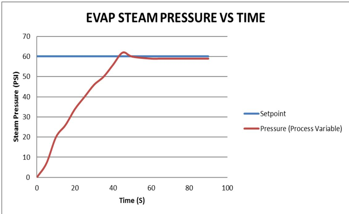
Figure 31: Behavior of Steam Pressure control loop over time
