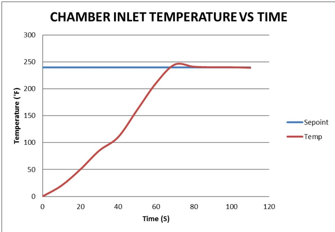
*Figure 33: Behavior of chamber Inlet Temperature control loop*
