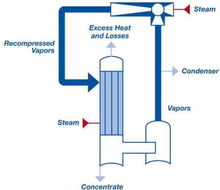
Figure 6: Diagram showing Calandria, Separator and TVR (Source: Niro Incorporated)
