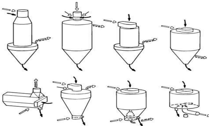
*Figure 17: Different designs of Dryer Chambers (Source: Vagn Westergaard, 2001)*
