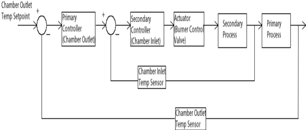
Figure 29: Block diagram showing chamber inlet and outlet temperature cascade loop
