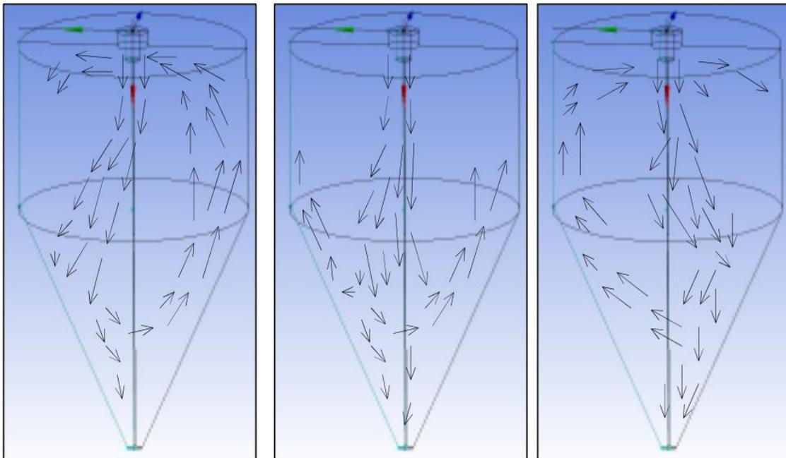
*Figure 16: Illustration of long term scale fluctuation focusing on the deflection of central air supply (Source: Arun Mujumdar, 2010)*
