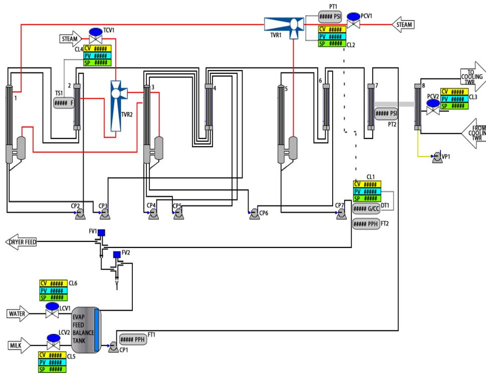
Figure 28: Dotted lines show Cascade between Steam Pressure and Density loops. Grey lines show sensor tied to each loop respectively.
