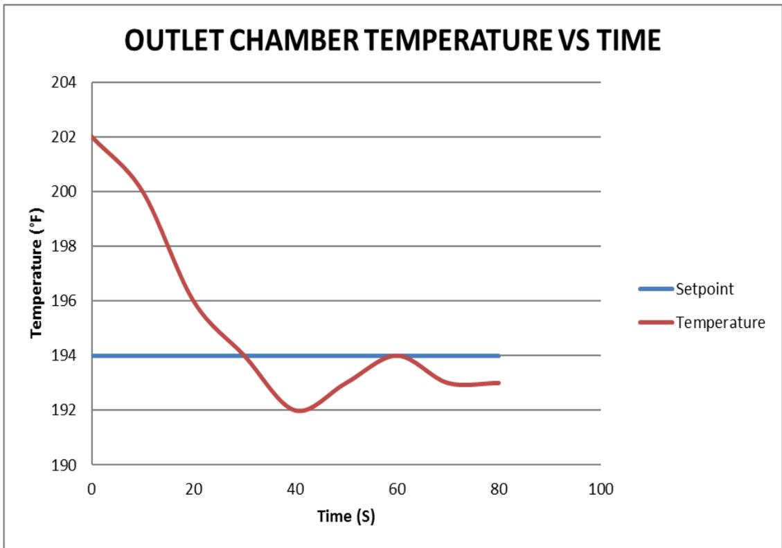
Figure 34: Behavior of Chamber Outlet Temperature loop during transition to product phase
