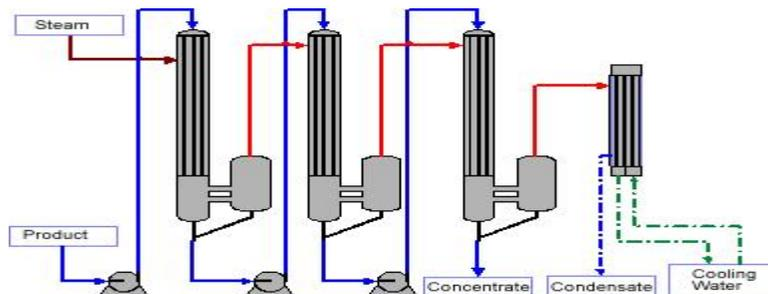
Figure 10: Multiple effect evaporator plant layout (Source: GEA Group AG, 2013)
