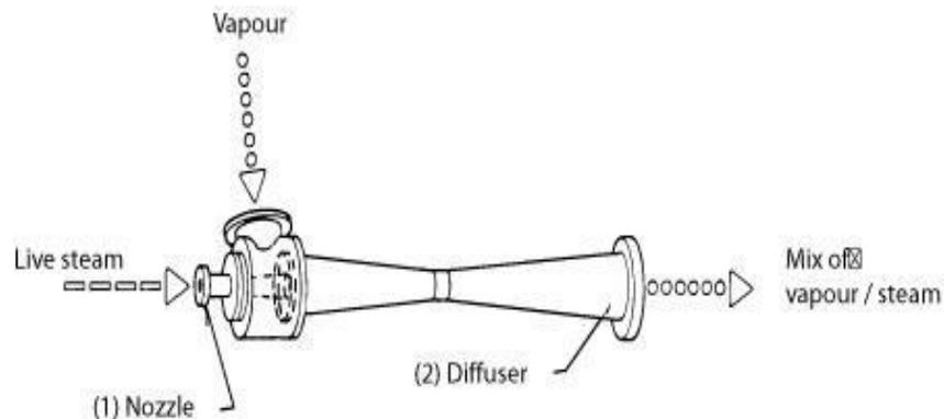
*Figure 5: Diagram of TVR showing Steam Nozzle, Vapor Inlet and Diffuser (Source: Niro Incorporated)*
