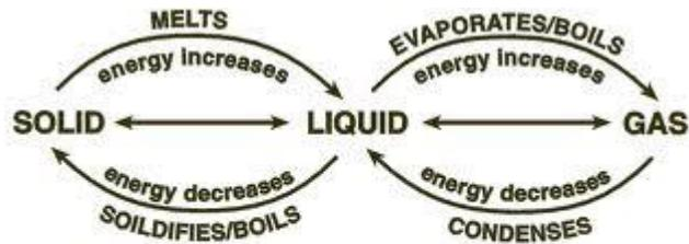
*Figure 2: A phase transition occurs when energy is added or removed from the system*
