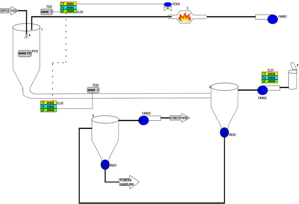
Figure 30: Dotted Line showing Cascade between Chamber Inlet and Outlet temperature loops. Grey lines show the sensor tied to each loop
