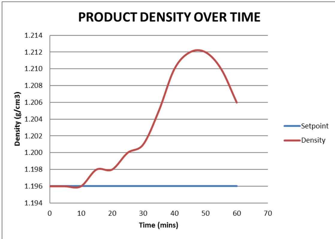
Figure 32: Density loop activated at  $1196 \text{ Kg/m}^3$ . Density Oscillates between  $1196 \text{ Kg/m}^3$  and  $1212 \text{ Kg/m}^3$
