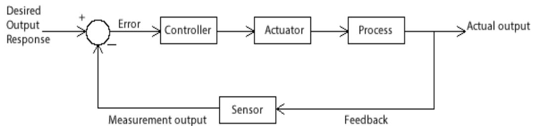
Figure 21: Closed loop control system
