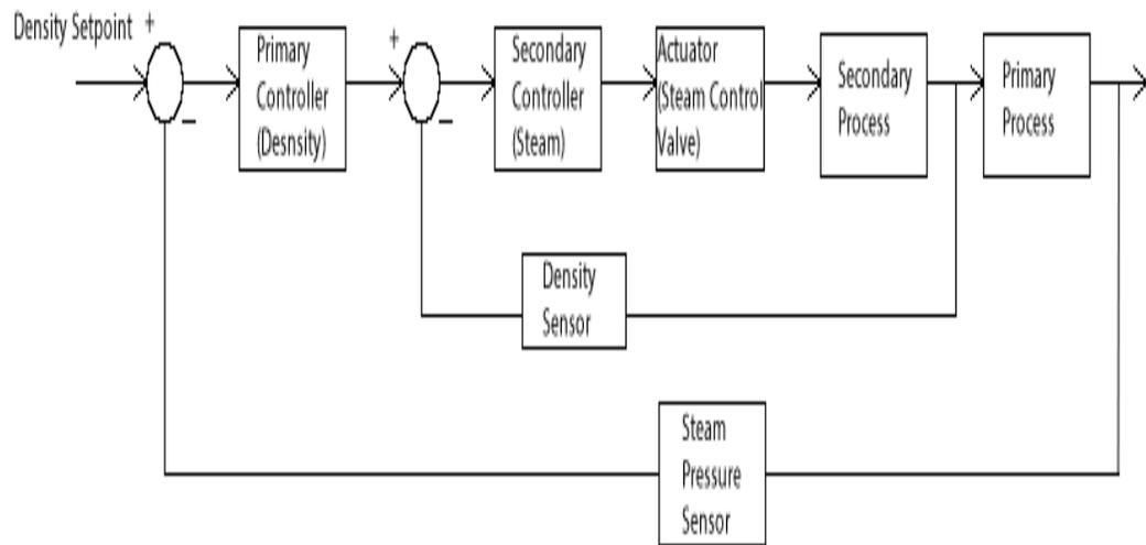
Figure 27: Steam pressure and density cascade loop block diagram
