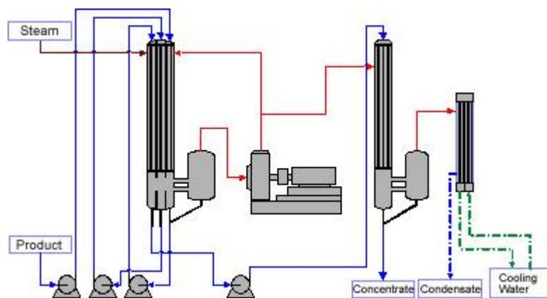
Figure 12: A 2 effect Evaporator plant layout with a Mechanical Vapor Recompressor (Source: GEA Group AG, 2013)
