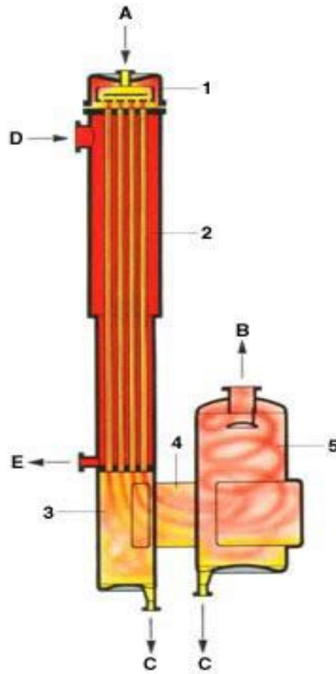
Figure 4: Calandria with heating tubes and separator (Source: Niro Incorporated)
