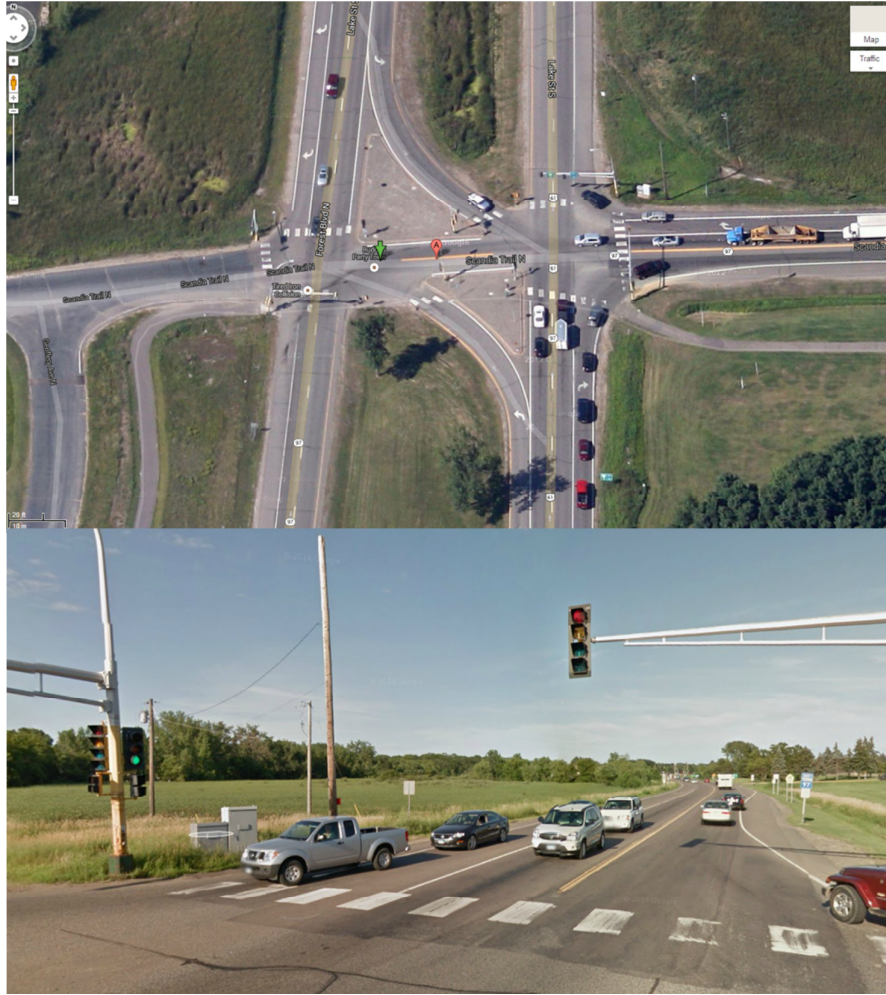
Figure 4-2. The site plan and the street view of a LT crash location with a 4-section special operation.
