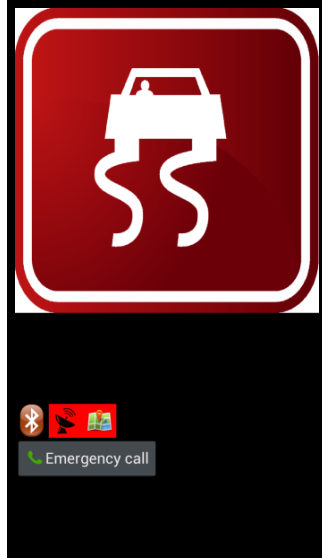
Figure 4. Excessive maneuver visual warning used for braking, turning, and acceleration events.
