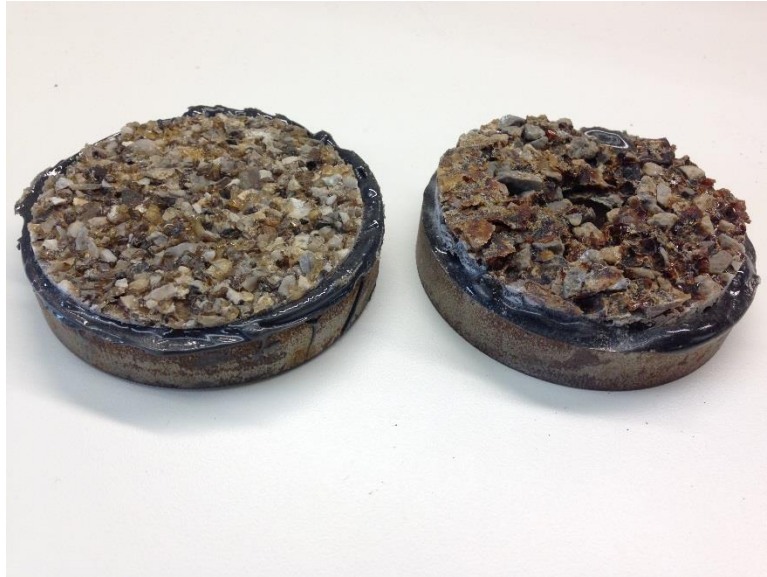
Figure 70: Comparison of Poly-Carb with Flint (Left) and SafeLane Torque Removal Samples
