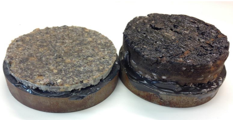
Figure 53: System Thickness Comparison. Left: Poly-Carb System, Right: Novachip System
