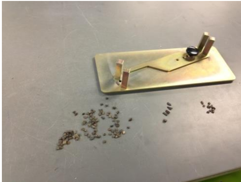
Figure 15: Flat/Elongation Measuring Equipment with Sorted Aggregate
