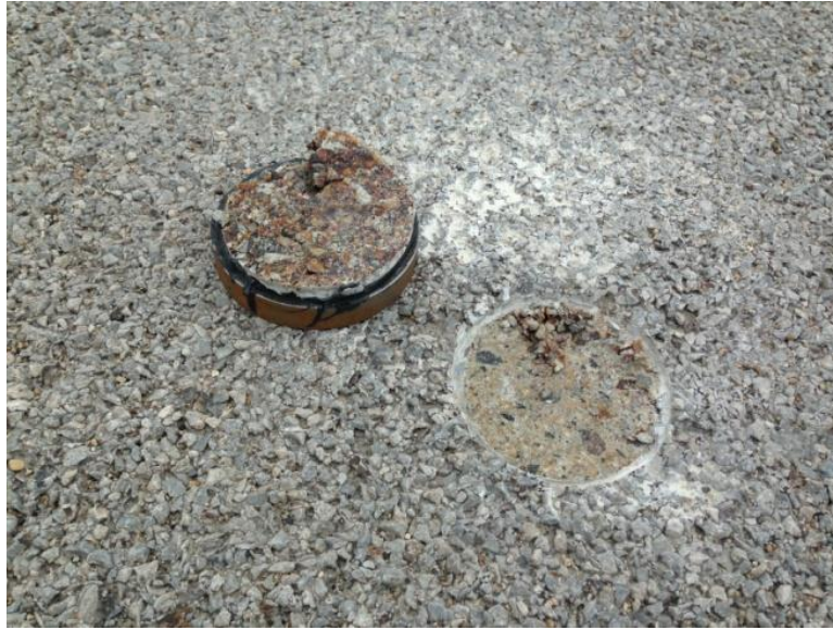
Figure 57: Plate with Debonded Overlay (Br 14810)
