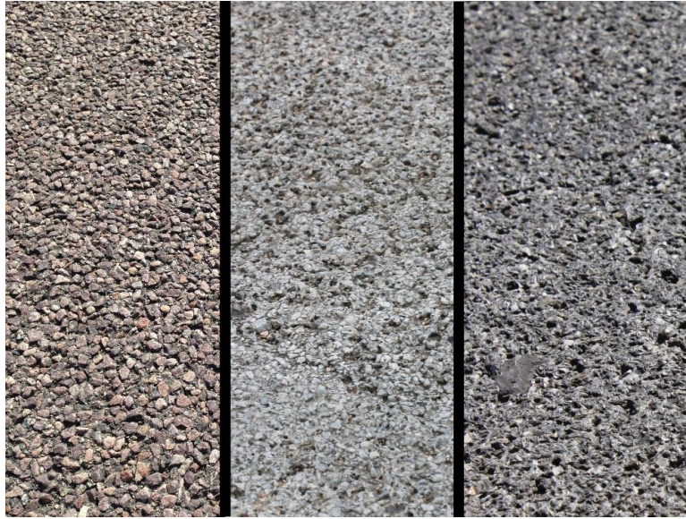
Figure 39: Comparison of Loss of Aggregate between Novachip (Left), SafeLane (Middle), and Poly-Carb (Right) Systems
