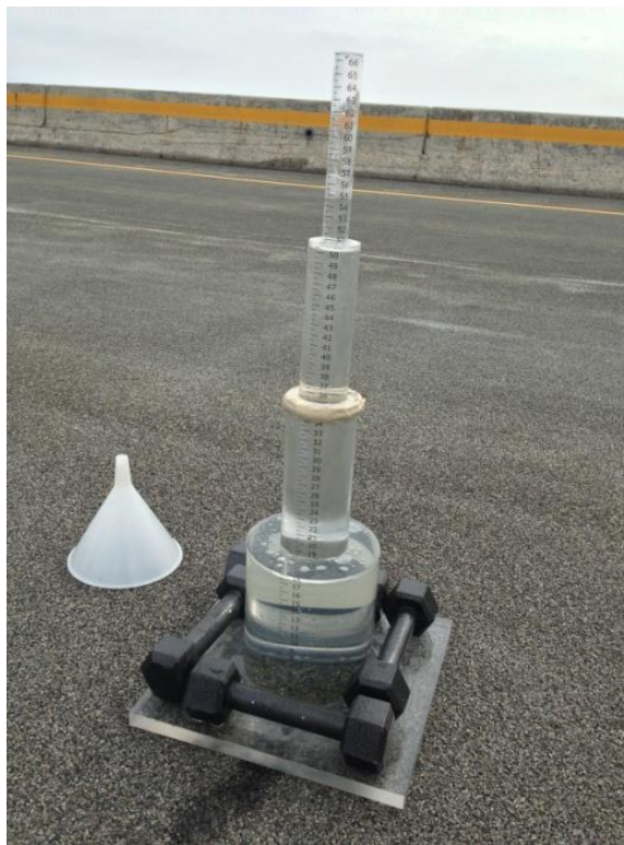
Figure 58: Permeability Test over Cracked Overlay (Br 9823)
