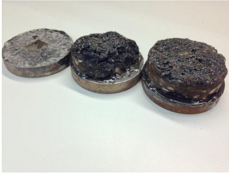
Figure 68: Various Degree of Removal Including "No Removal" (Left), "Partial Removal" (Middle), and "Total Removal" (Right)
