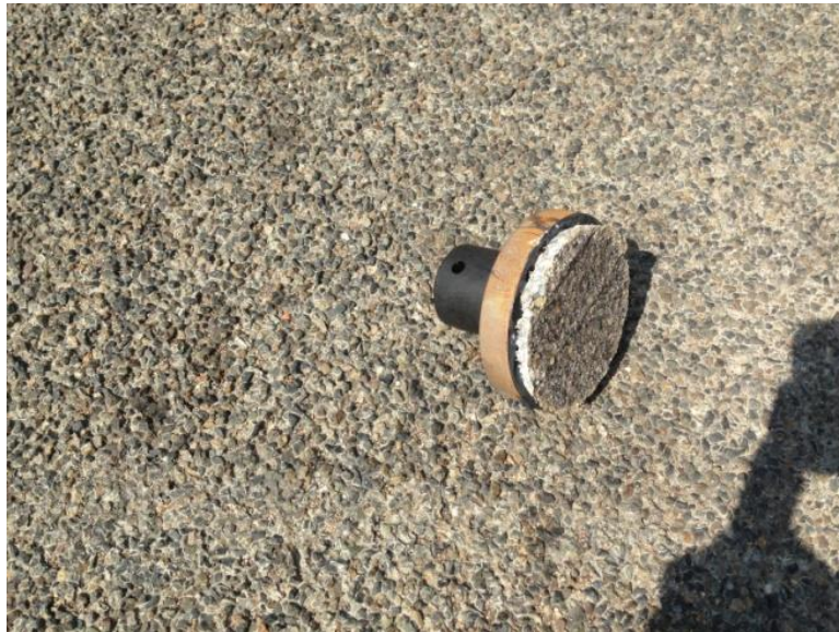
Figure 56: Plate with Debonded Overlay (Br 9036)
