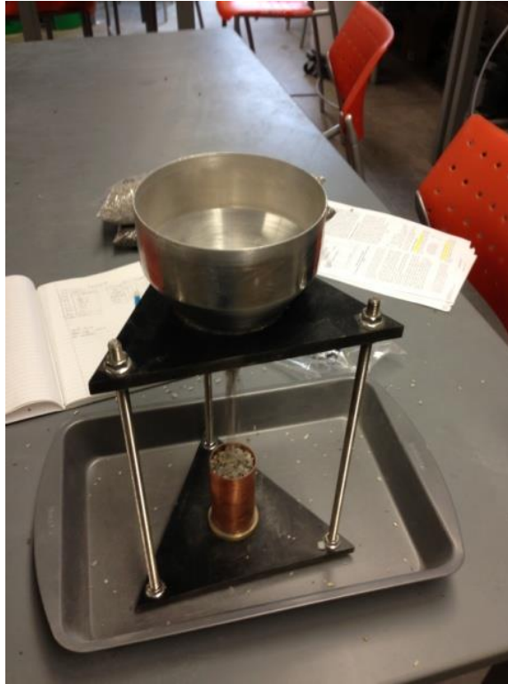
Figure 14: Aggregate Sample Falling into Calibrated Cylinder
