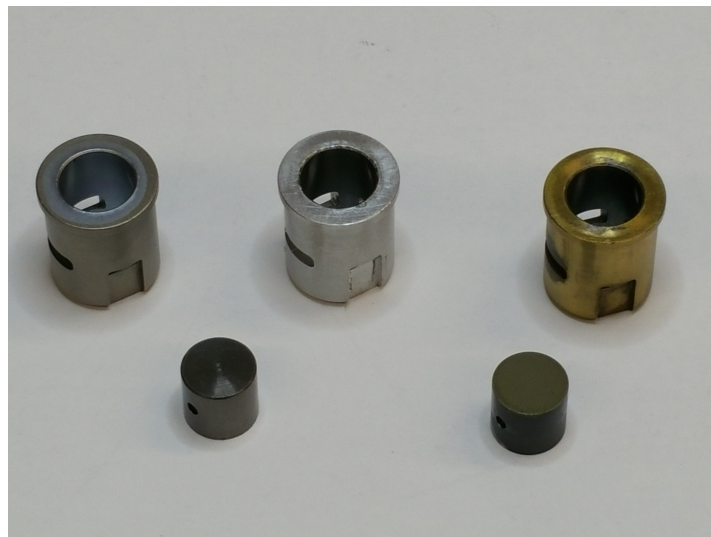
Figure 3.10: Various pistons and cylinder liners. Top, left to right: brass liner with nickel-Teflon coating, aluminum liner with chrome plating, brass liner with chrome plating. Bottom, left to right: aluminum piston with nickel-Teflon coating, stock aluminum piston with commercial low friction coating.
