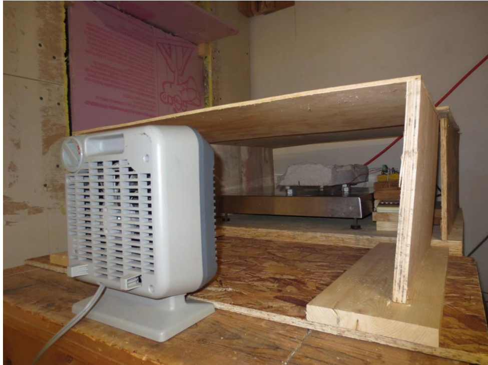
Figure 4-5: Drying Enclosure for Calibration CMU
