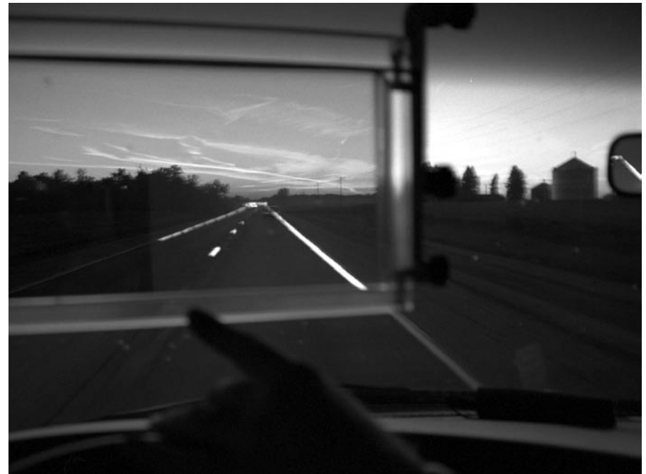
The HUD, shown here on a vehicle at dusk, can help drivers “see” the roadway when low-visibility might otherwise obscure it.
