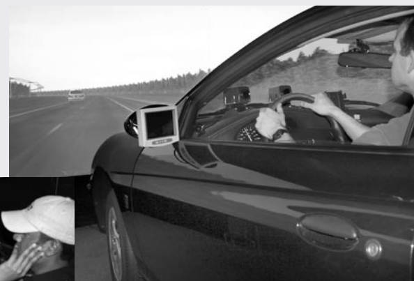
Data are collected by two cameras mounted on the dashboard (above), while research assistant Praveen Balachandran (left) monitors where the driver is looking.
