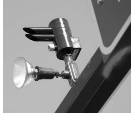
Sensors mounted on or near traffic signals can alter a signal's timing cycle in response to an approaching emergency vehicle.
