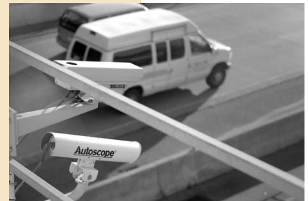
Portable monitoring stations transmit freeway traffic data to the ITS Lab.
