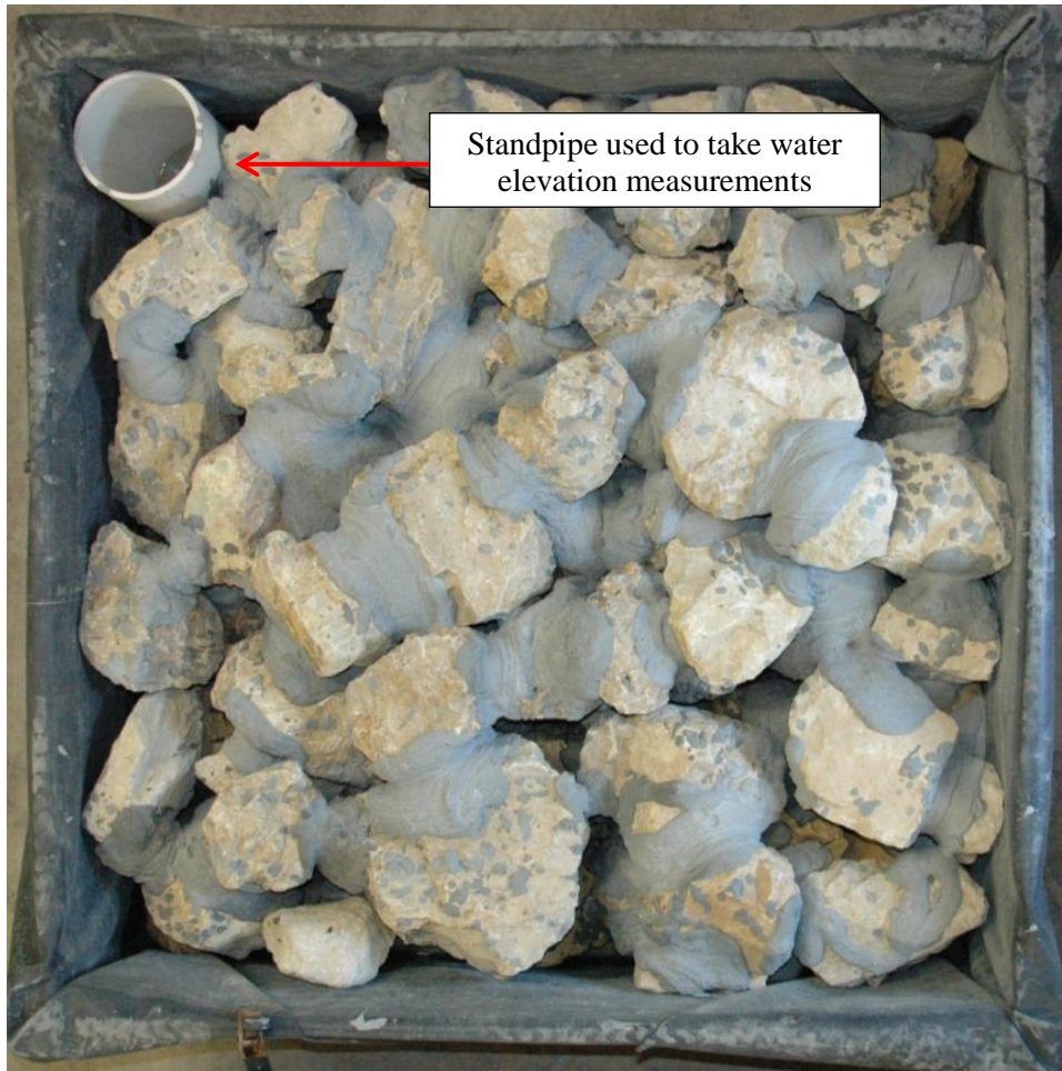
Figure 4.3. Image of a box after filled with riprap and grouted.
