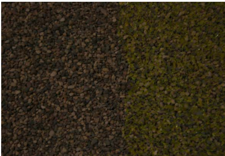
Figure 5.16. Side by side comparison of pea gravel surface with and without hot glue "grout".
