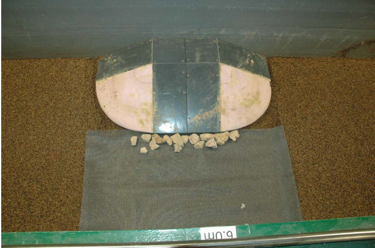
Figure 5.4. Image showing the setup for a spill through abutment experiment in the Tilting Bed Flume. The image shows the filter material, the model riprap material, and Model 1 Abutment.
