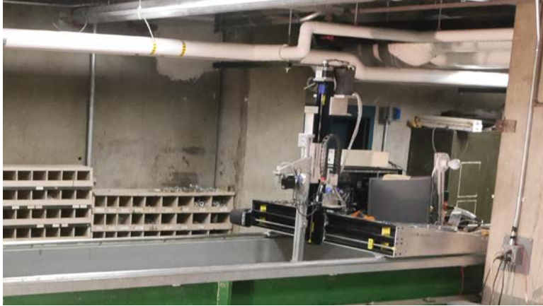
Figure 5.5. Tilting Bed Flume data carriage used to take precision velocity and topographic scans.
