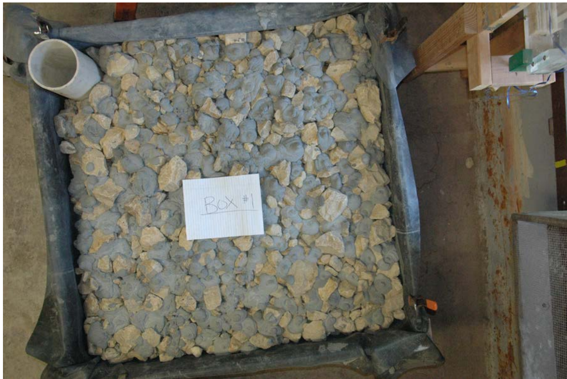
Figure 4.1. Example Out-of-Flume test box configuration.
