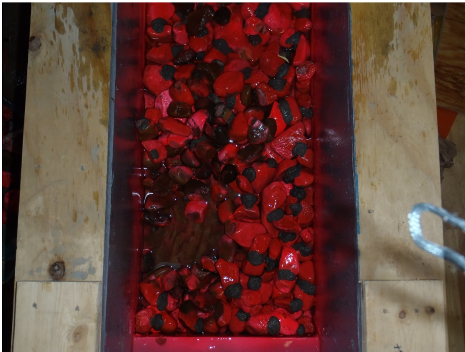
Figure 6.26. Post-Run 10, 2-inch river rock with half of the recommended grout.
