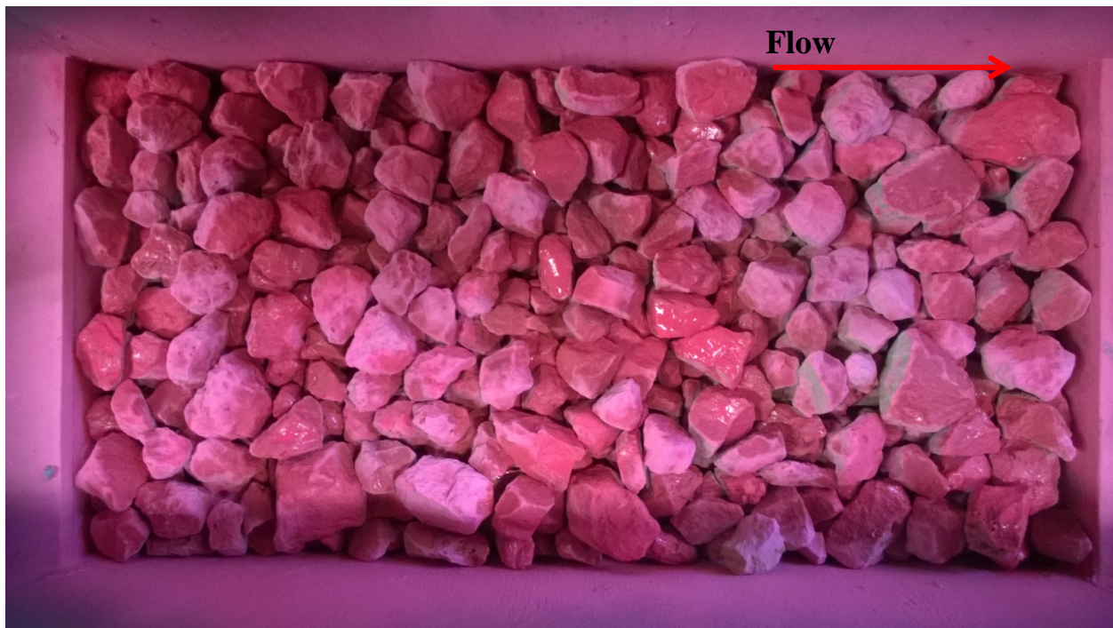
Figure 6.8. Pre-Run 1, 2-inch angular gravel with no grout.
