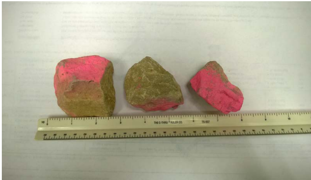
Figure 6.2. 2-inch angular gravel.
