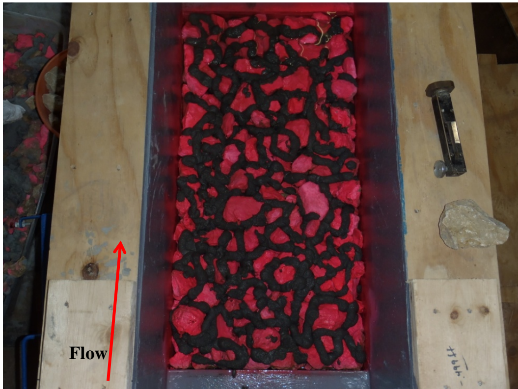
Figure 6.11. Post-Run 2, 2-inch angular gravel with grout placed according to MnDOT guidelines.
