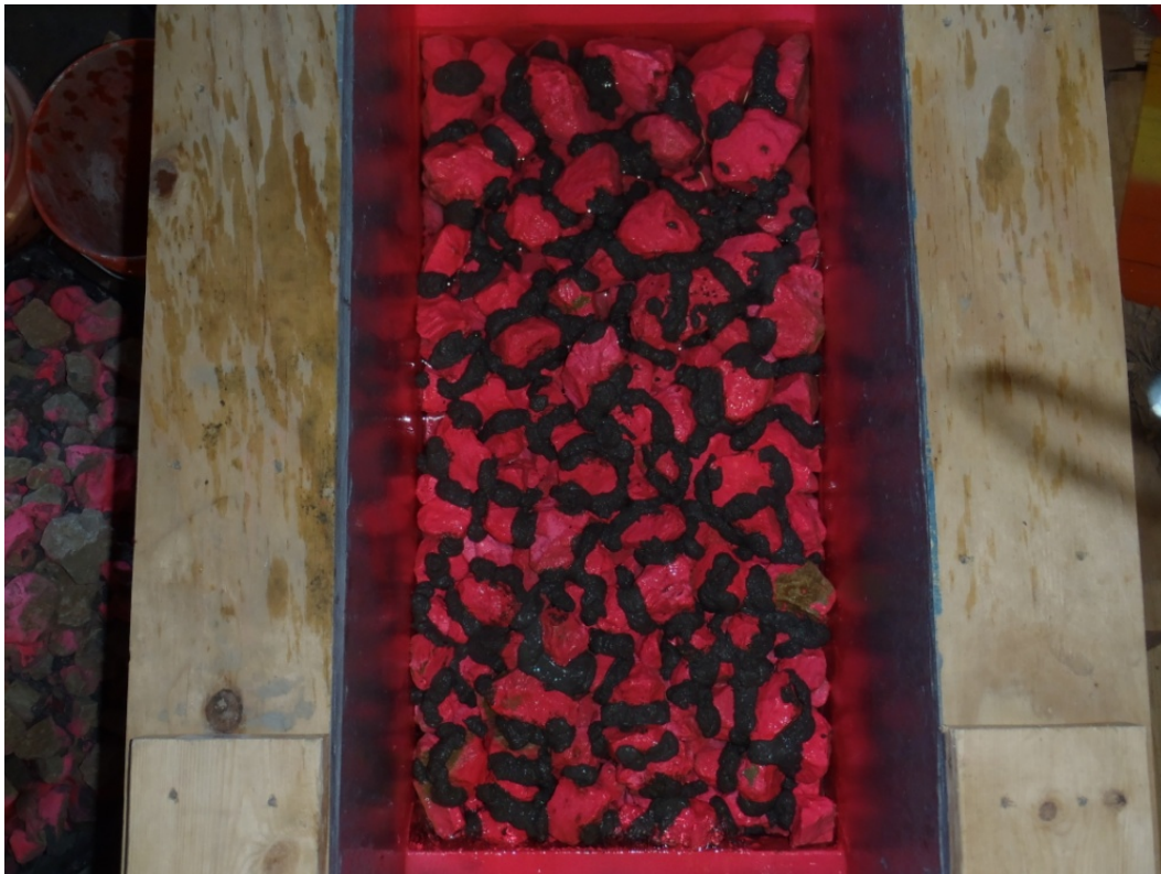
Figure 6.17. Post-Run 5, 2-inch angular gravel with half recommended grout.
