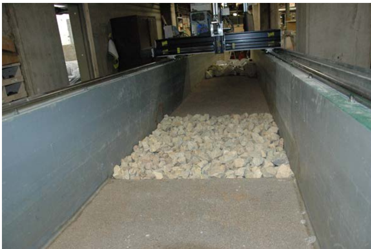
Figure 5.19. Plane bed configuration, riprap only.
