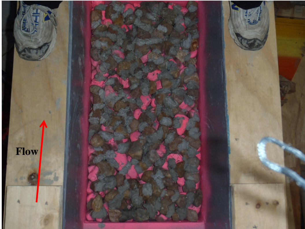
Figure 6.22. Pre-Run 8, 2-inch river rock with grout placed according to MnDOT guidelines.
