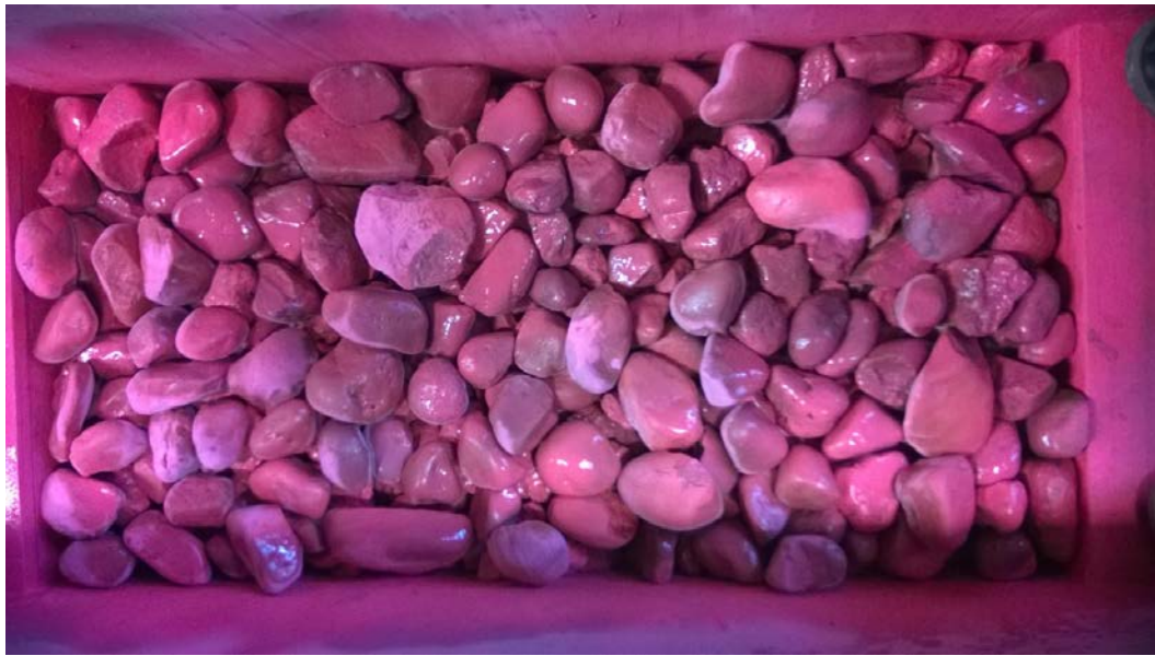
Figure 6.18. Pre-Run 6, 2-inch river rock with no grout.
