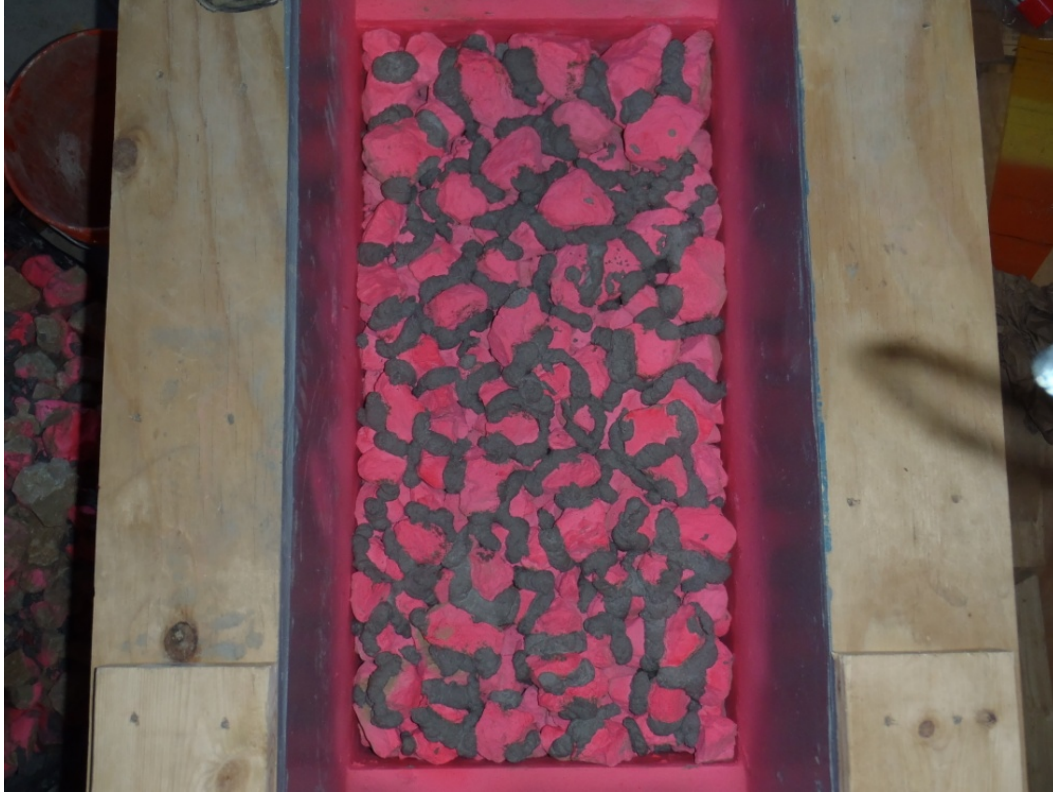
Figure 6.16. Pre-Run 5, 2-inch angular gravel with half recommended grout.
