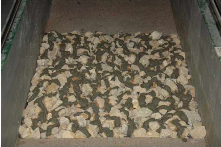
Figure 5.20. Plane bed configuration, matrix riprap.
