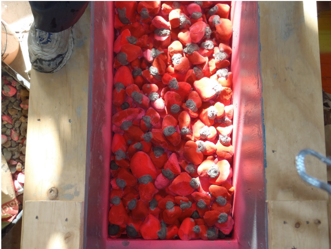
Figure 6.24. Pre-Run 9, 2-inch river rock with half of the recommended grout.
