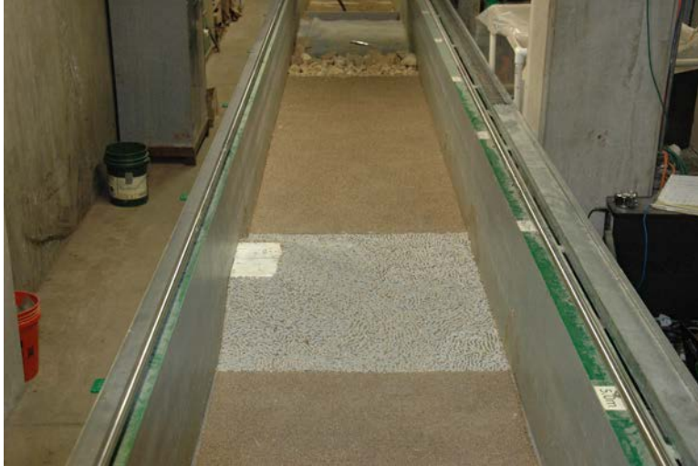
Figure 5.18. Image of Quickcrete matrix riprap within the Tilting Bed Flume.
