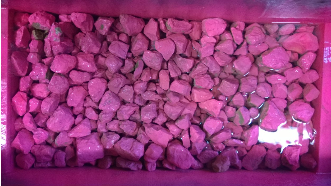
Figure 6.9. Post-Run 1, 2-inch angular gravel with no grout.
