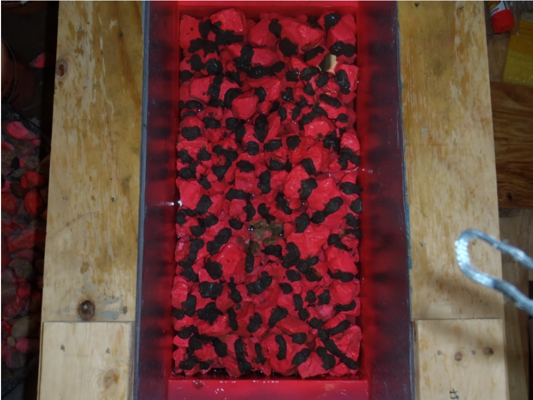
Figure 6.15. Post-Run 4, 2-inch angular gravel with half recommended grout.
