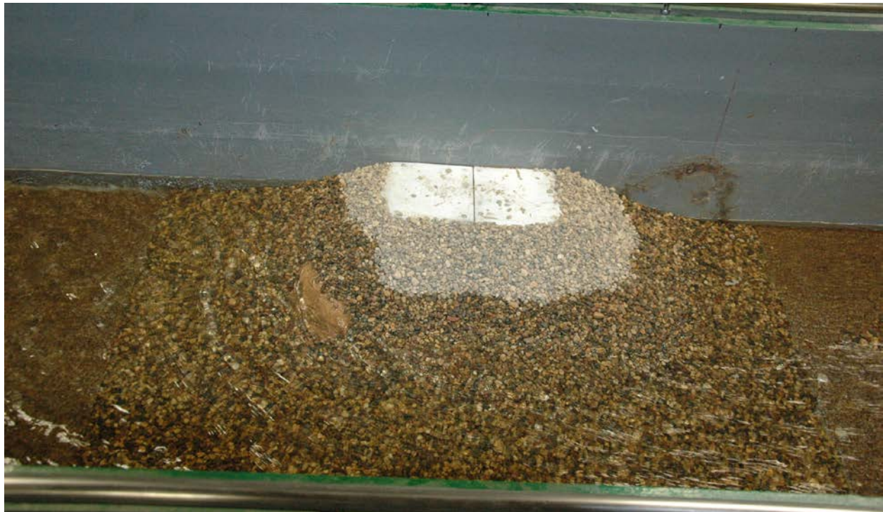
Figure 5.12. Flume setup for Model 1 with pea gravel.
