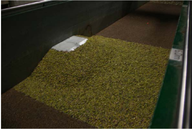
Figure 5.15. Hot glue applied to finished riprap surface.
