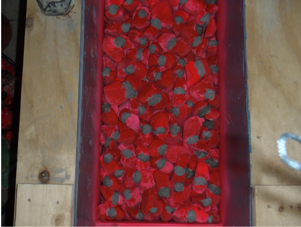
Figure 6.25. Pre-Run 10, 2-inch river rock with half of the recommended grout.
