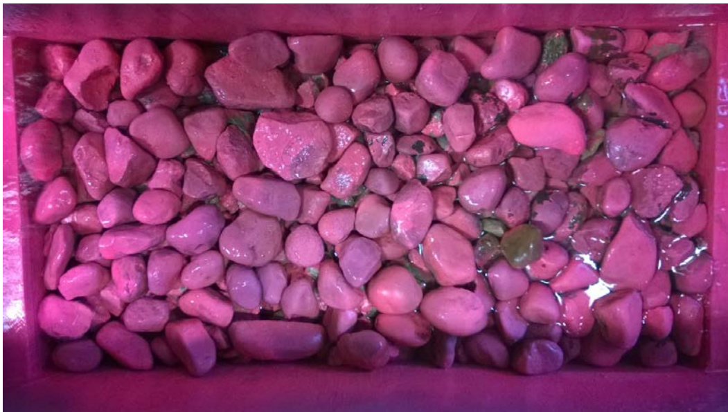
Figure 6.19. Post-Run 6, 2-inch river rock with no grout.
