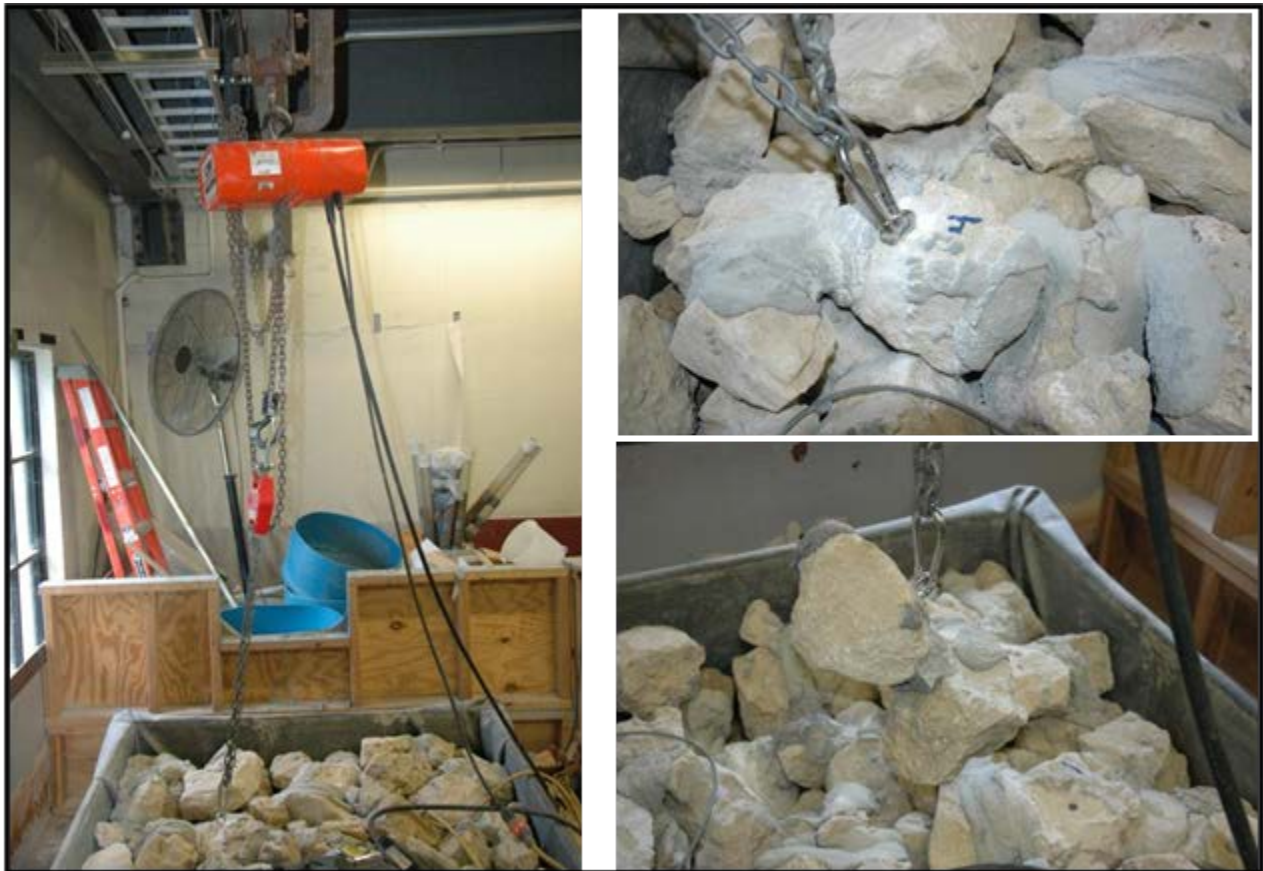
Figure 4.13. Mechanical pull test apparatus and anchoring system.
