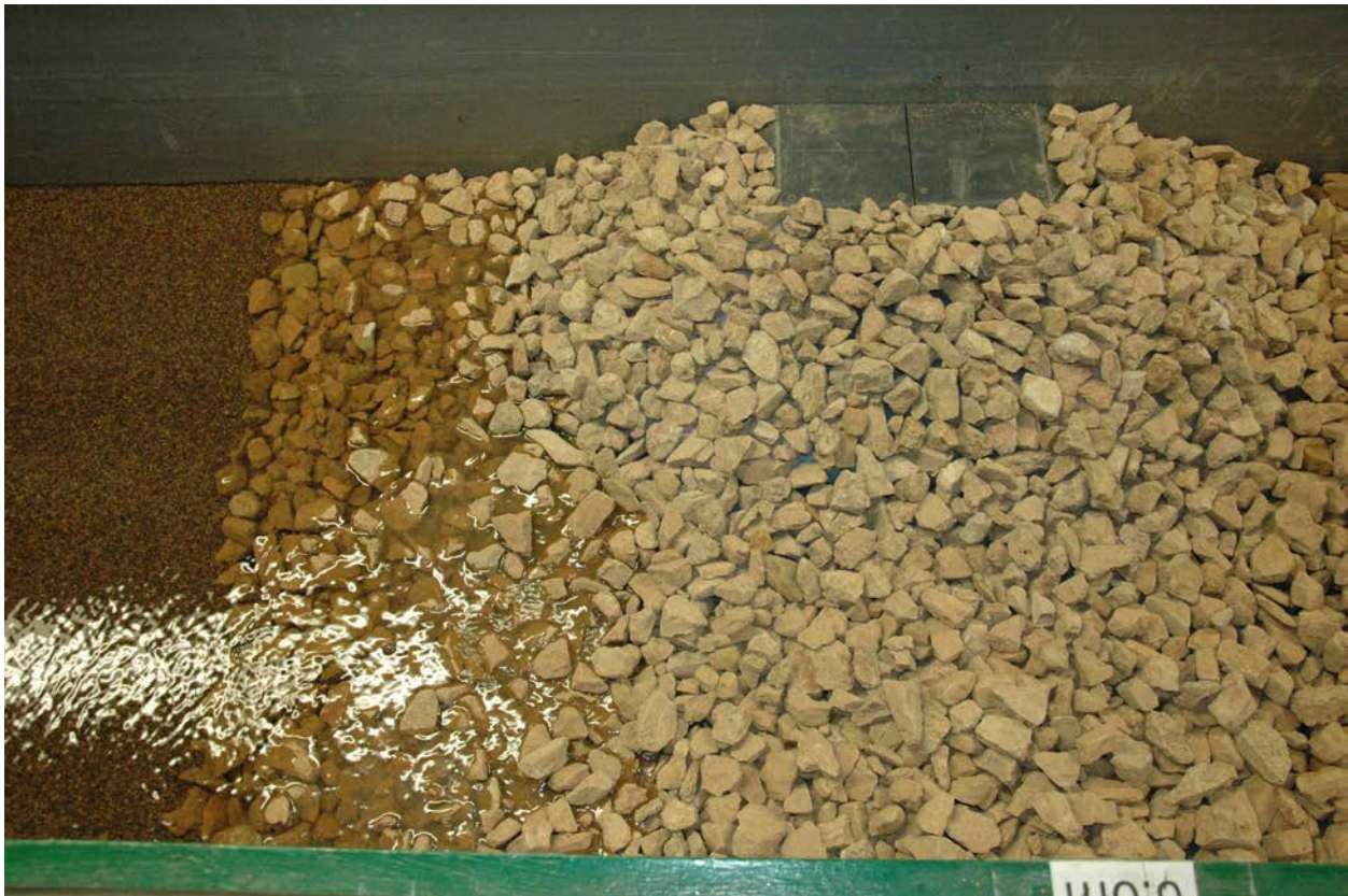
Figure 5.6. Photograph of the abutment with 25 mm riprap material.
