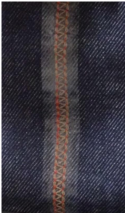
Figure 5.3 Insulation by Fusing technique: a strip of bonding film is fused on the stitched sensor
