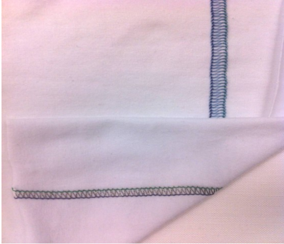
Figure 4.4. Top-thread sensor horizontally folded on the left in gray, bottom-thread cover vertically on the right in blue on elastomeric fabric
