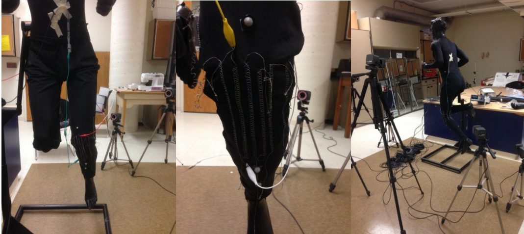
Figure 6.3. From left-to-right: Bottom-thread coverstitched sensors stitched on the frontal side of the left knee of an animatronic mannequin. Alligator clip connection - zoom. Experiment Setup
