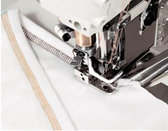
Figure 4.3. Juki MF-7723 high-speed, flat-bed coverstitch machine
