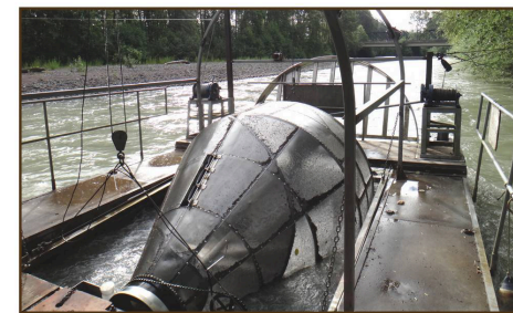
A screw trap near the Main Street Bridge churns away on the Puyallup River.
