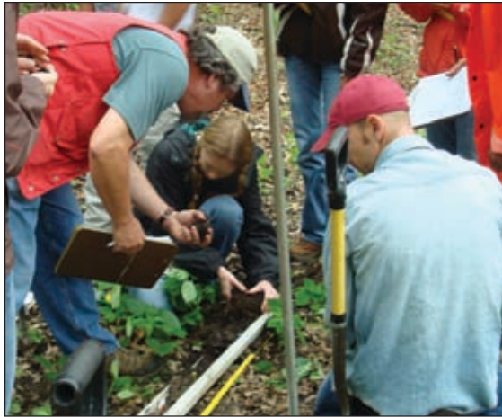
Wetland delineation students learn how to profile soil. When profiling soil, students must describe soil colors, distinguish soil horizons, and differentiate among loamy, clay, and sandy textures.
