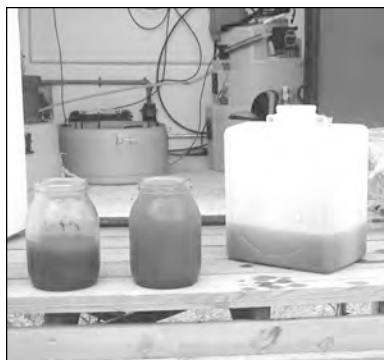
Le Sueur River Station: flow composite samples ready for splitting between MCES and MDA after a May 2002 rain.
