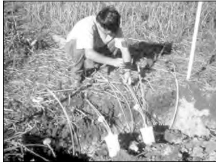
A student installs water quality samplers.
