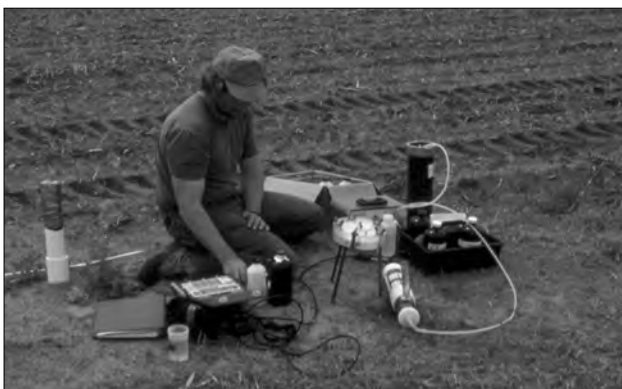
Dan Rosemore of the USGS collects groundwater samples from a study farm system.
