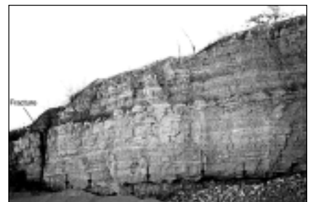
Typical example of large, interconnected, dissolution cavities arranged parallel to beds of dolostone in southeastern Minnesota. These cavities (arrows) are connected to the surface by a vertical fracture exposed along the quarry wall on the left side of the photo. Using a number of recently developed borehole geophysical techniques, recognition and predictability of these kinds of important groundwater conduits in deep, saturated subsurface conditions is now greatly enhanced.
